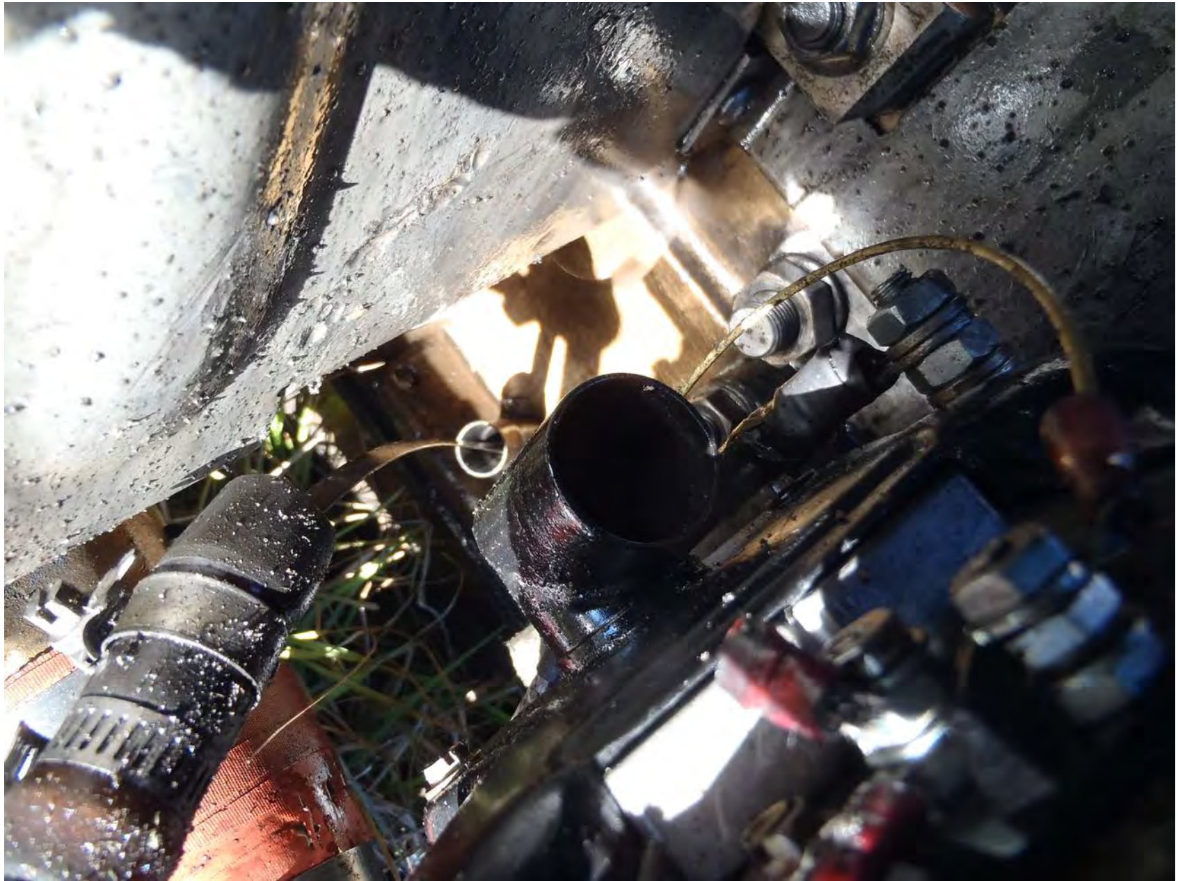
Photo 19 – Right Engine's Oil Gage Housing Extension
