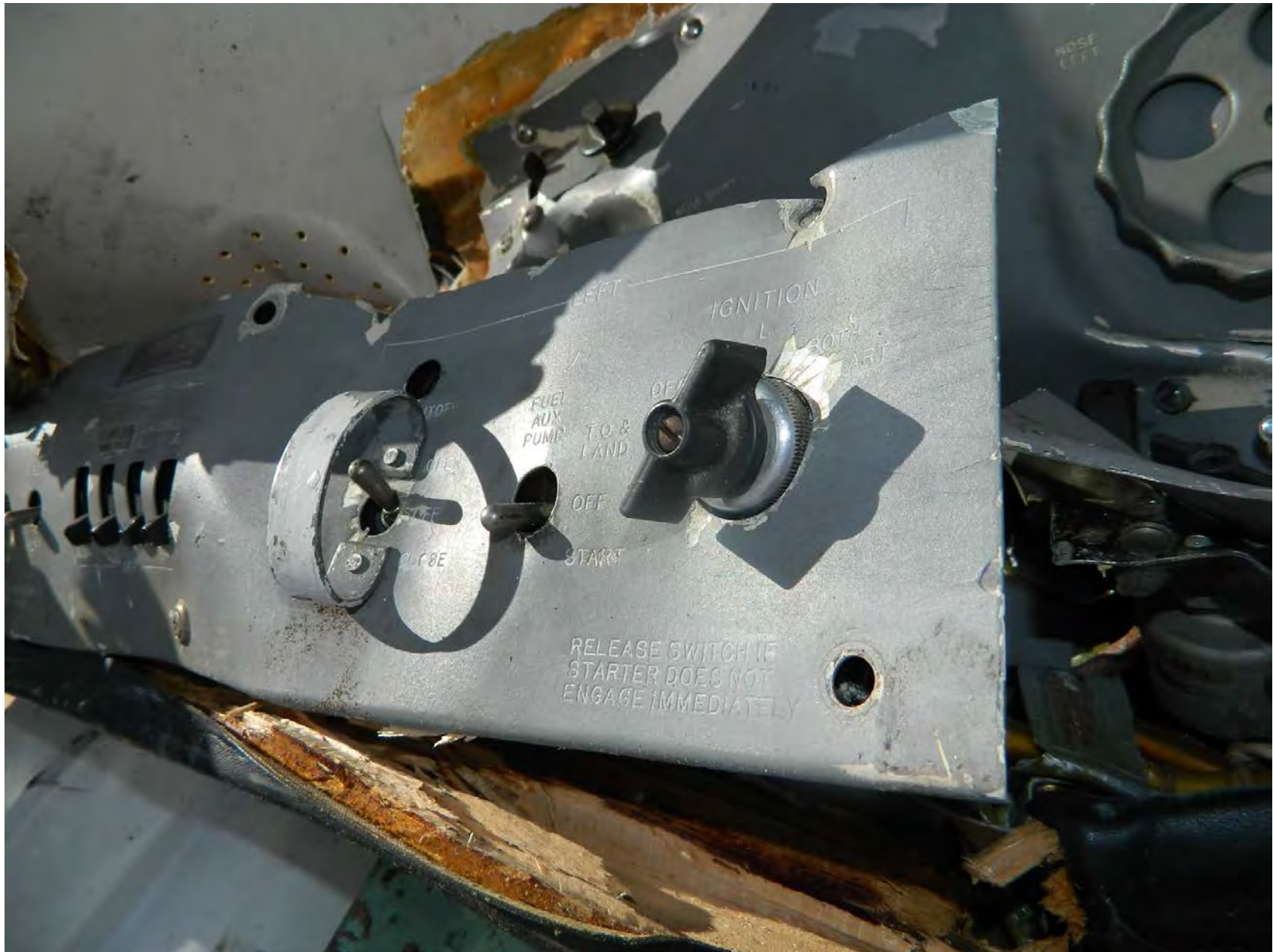
Photo 13 – Left Engine’s Fuel and Ignition Switches
