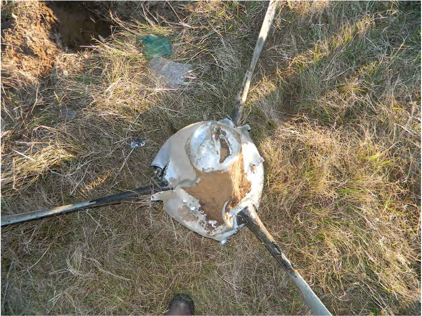
Photo 6 – Right Propeller After Extraction
