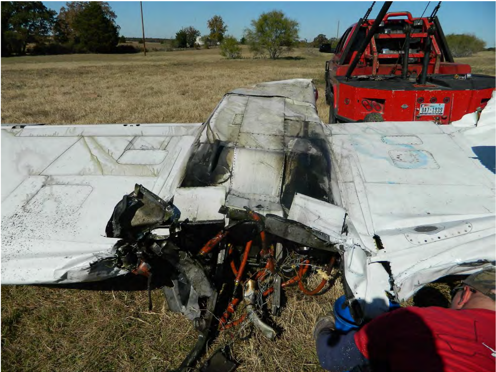
Photo 17 – Underside of Right Wing
