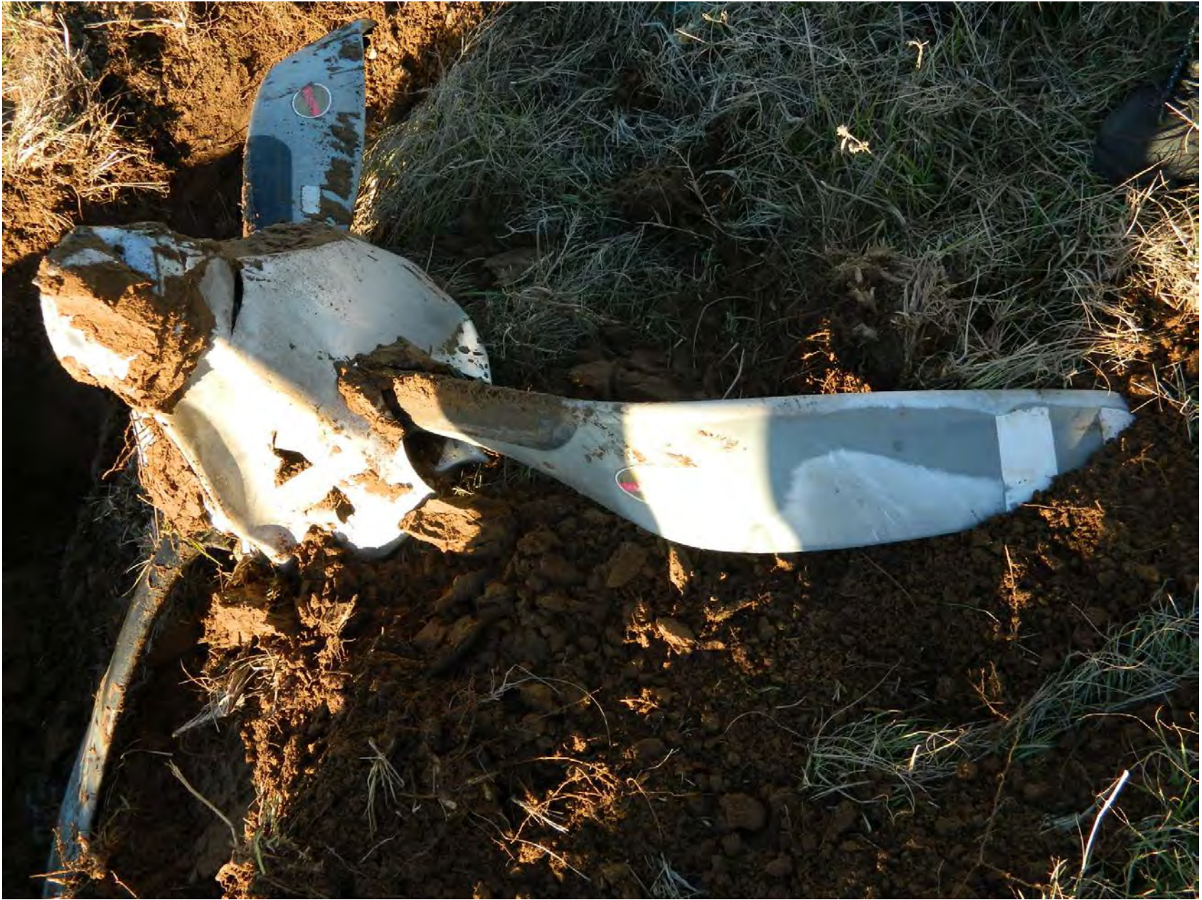
Photo 4 – Left Propeller After Extraction
