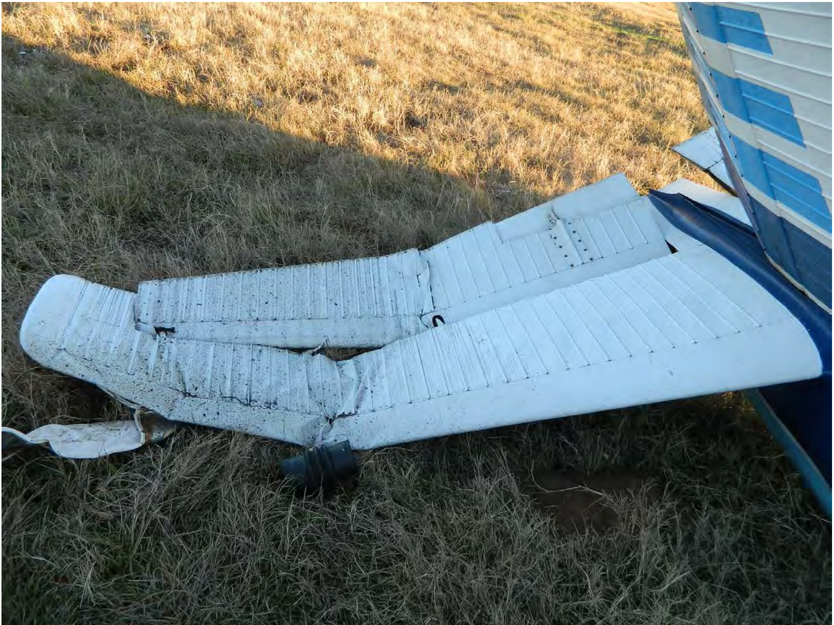
Photo 8 – Right Horizontal Stabilizer
