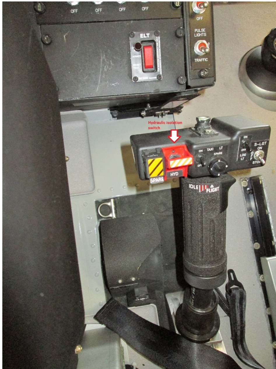
Photo 2 – Hydraulic isolation switch
