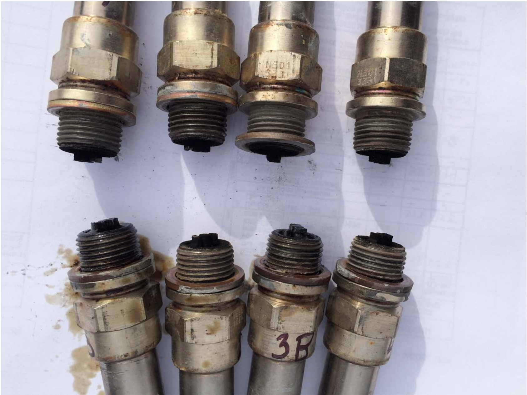
Photo 7 – Spark plugs displaying carbon fouling
