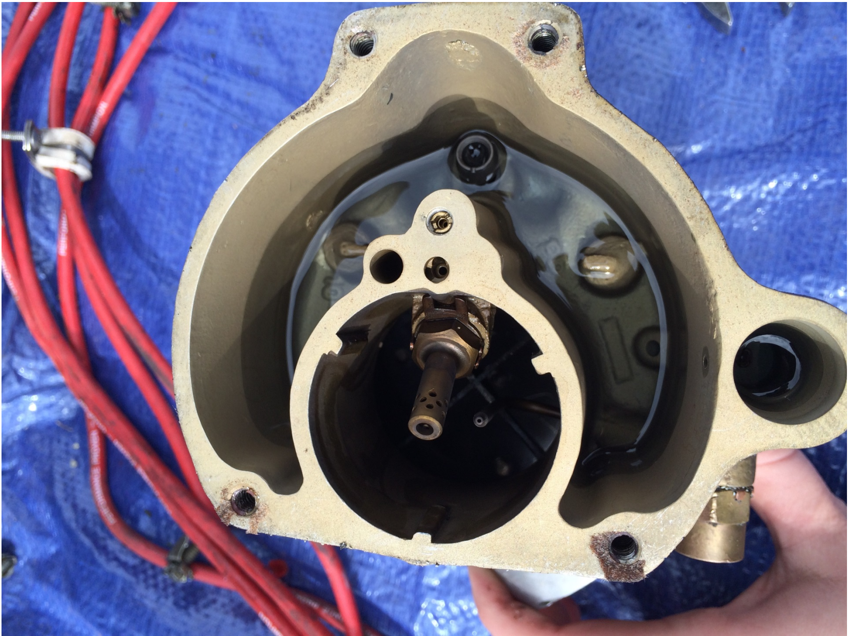
Photo 6 – Carburetor float bowl with fuel
