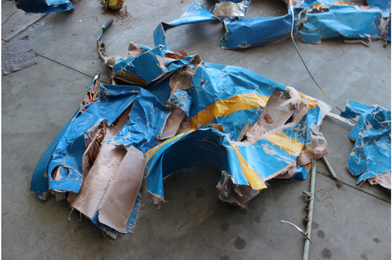
Figure 6: Impact damage to the left lower wing
