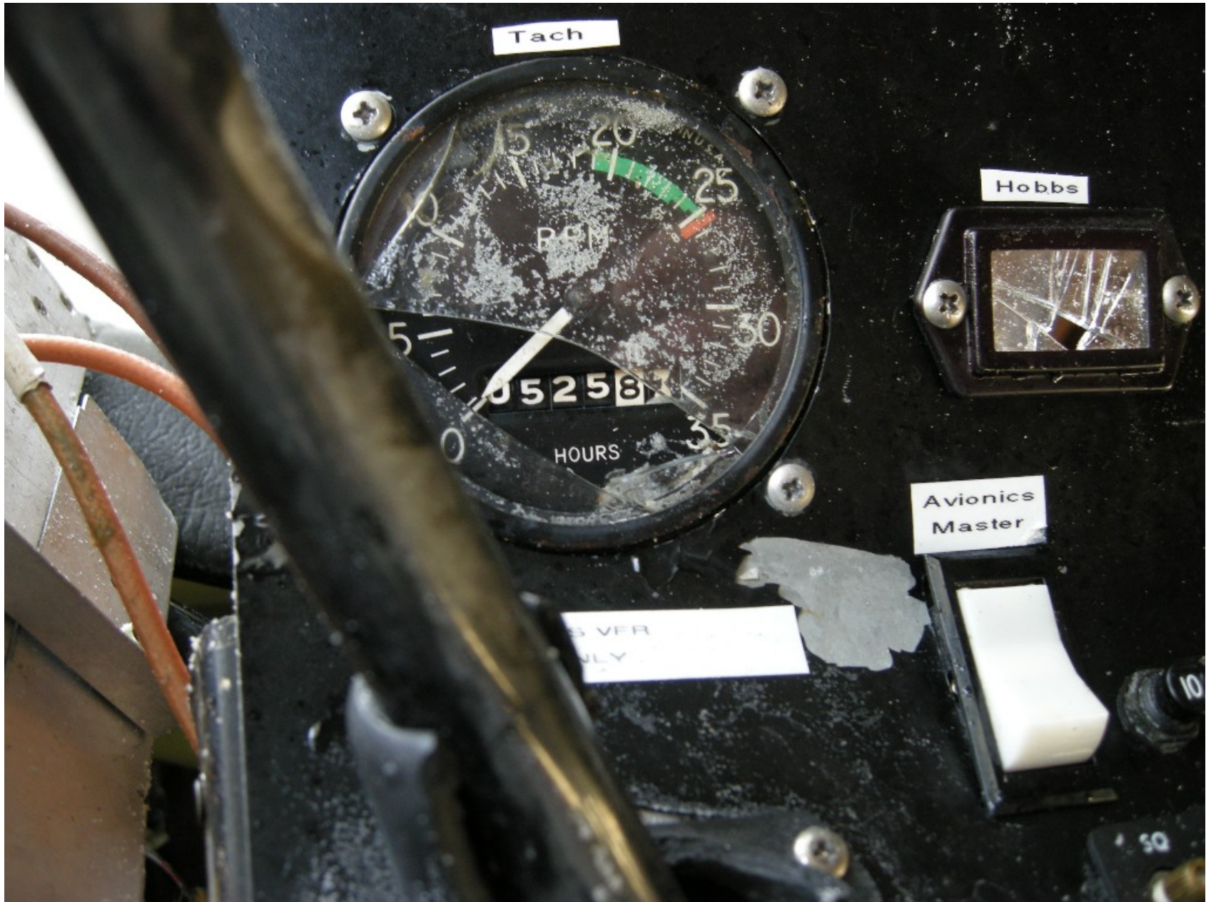
Photo 14 – Engine Tachometer (NTSB Photo)
