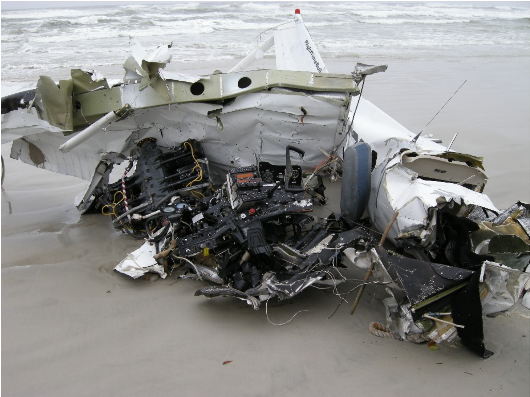
Photo 7 – Forward Fuselage (NTSB Photo)
