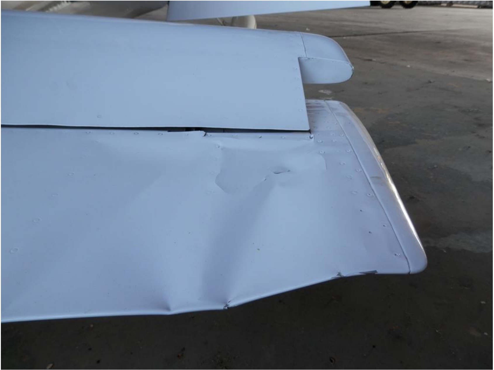
Photo 4 – Elevator damage (Courtesy of FAA)
