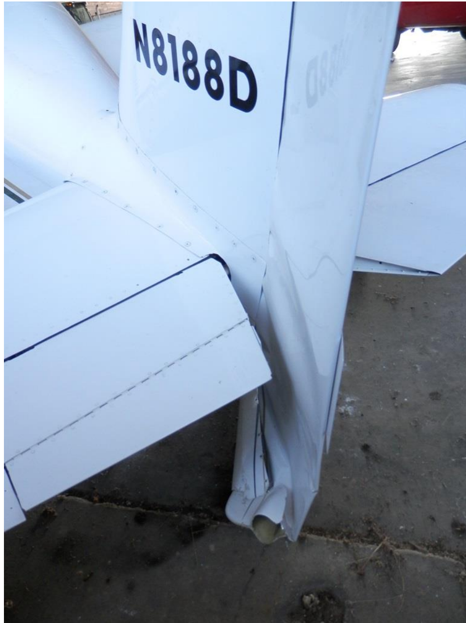
Photo 3 – Rudder damage (Courtesy of FAA)
