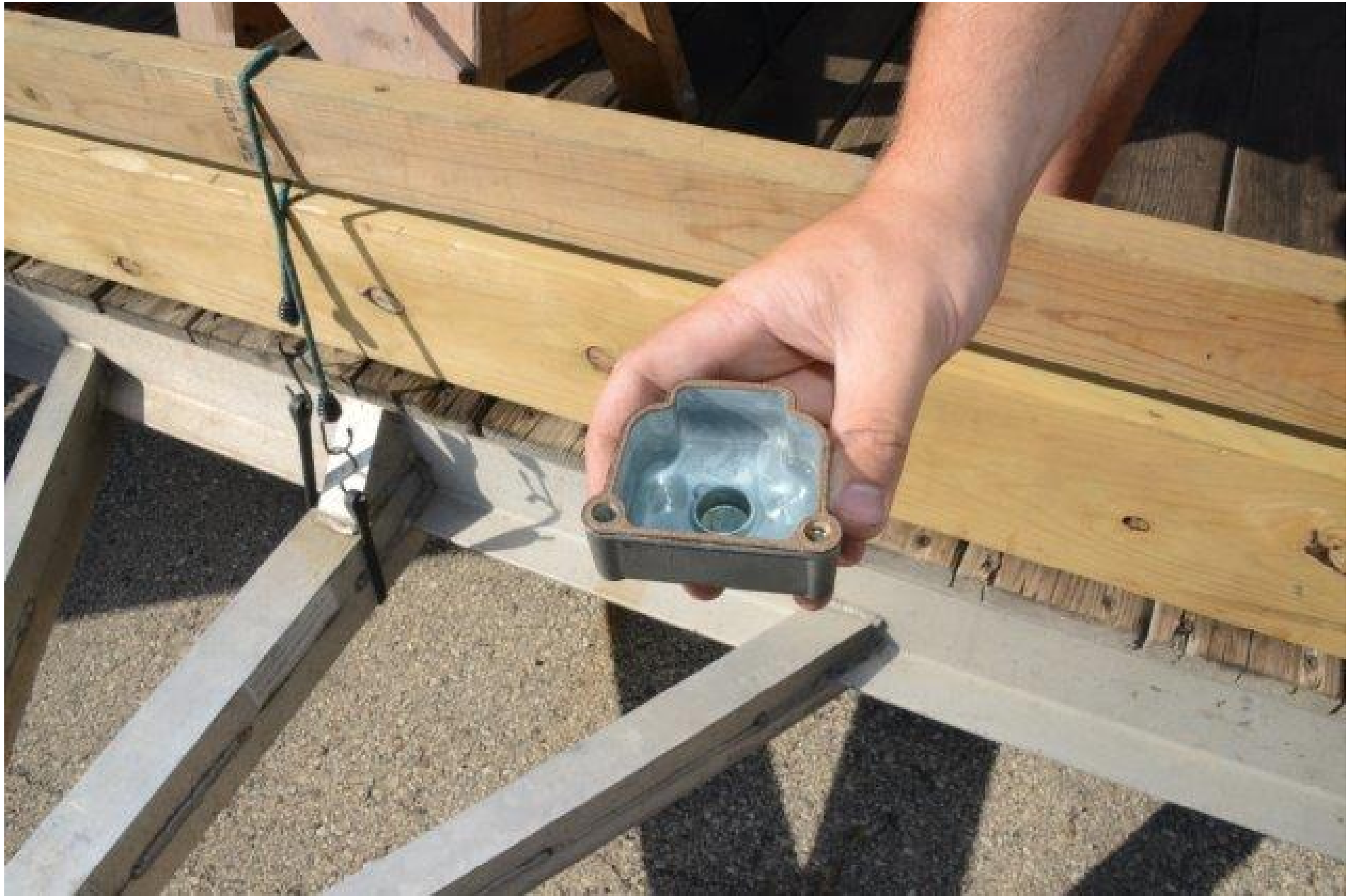
Photo 8 - View of the carburetor bowl with a blue liquid in it.
