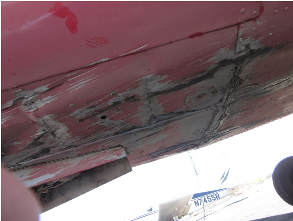
Figure 4: Belly Damage just aft of the Nose landing gear
