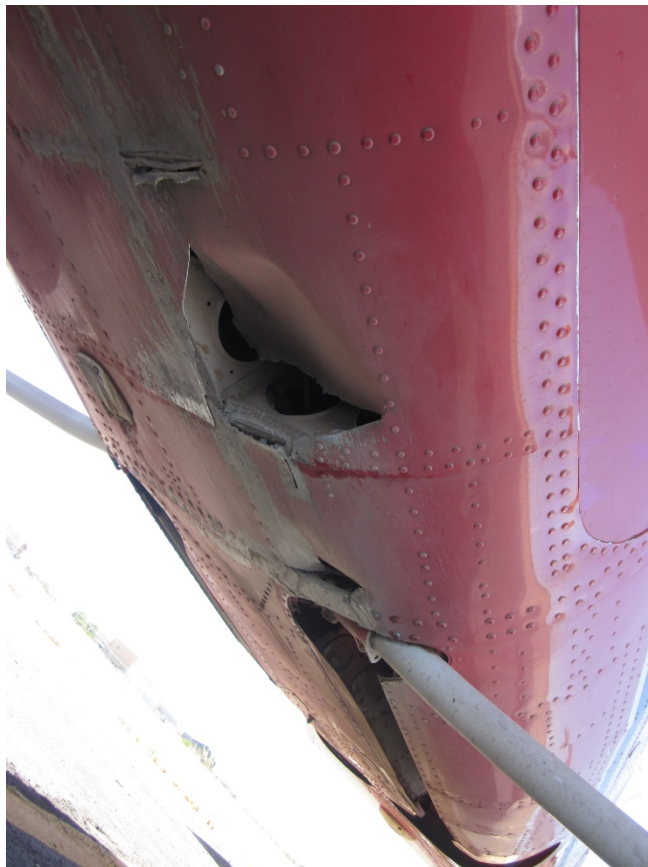
Figure 5: Lower Skin "hole" Damaging the Pressure Vessel
