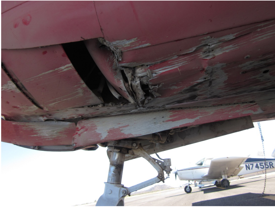
Figure 3: Belly Damage at the Nose Landing Gear
