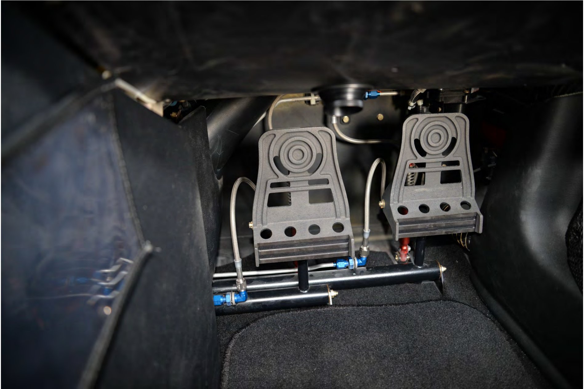
Photo 15 - View of the right-side rudder pedals.
