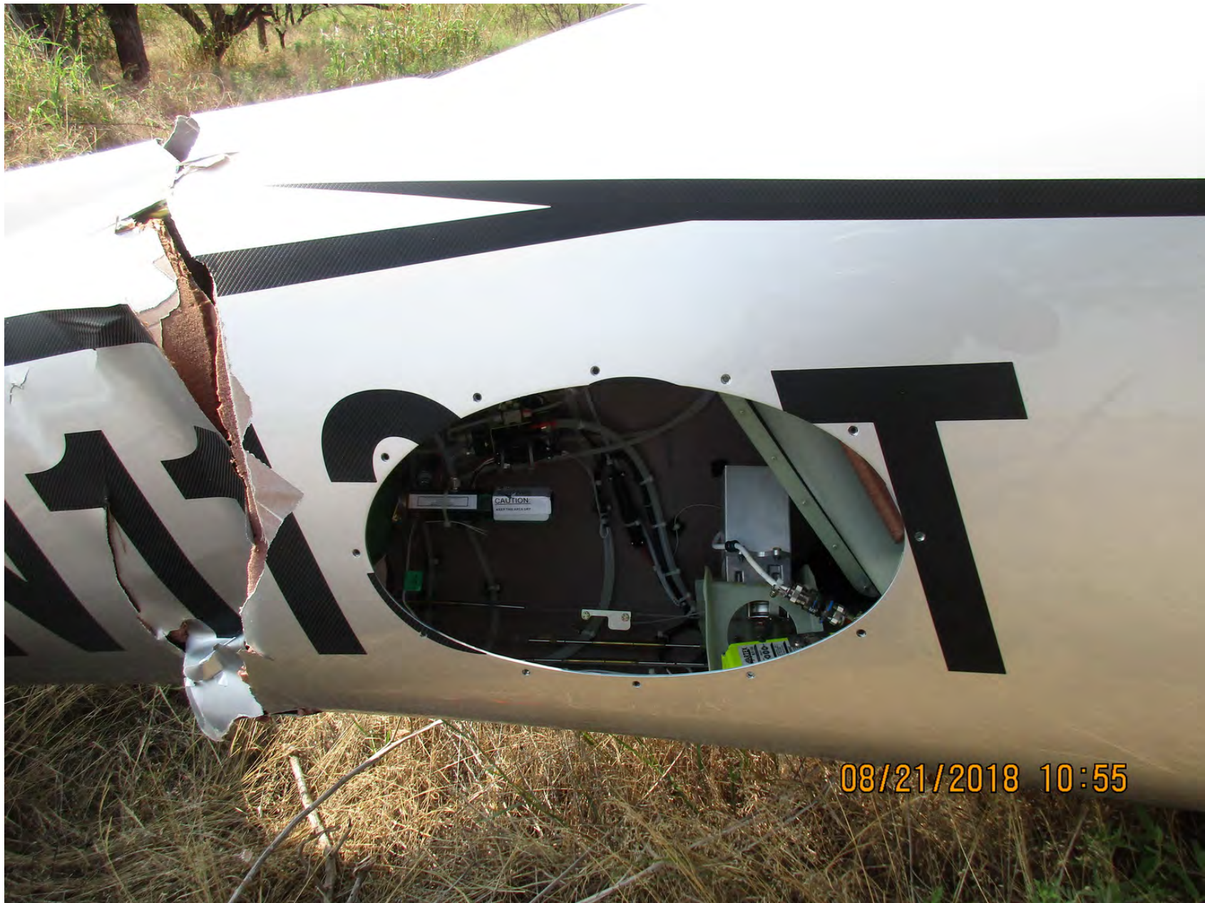
Photo 14 - View of an open fuselage panel. The yaw damper servo is inside the panel opening.
