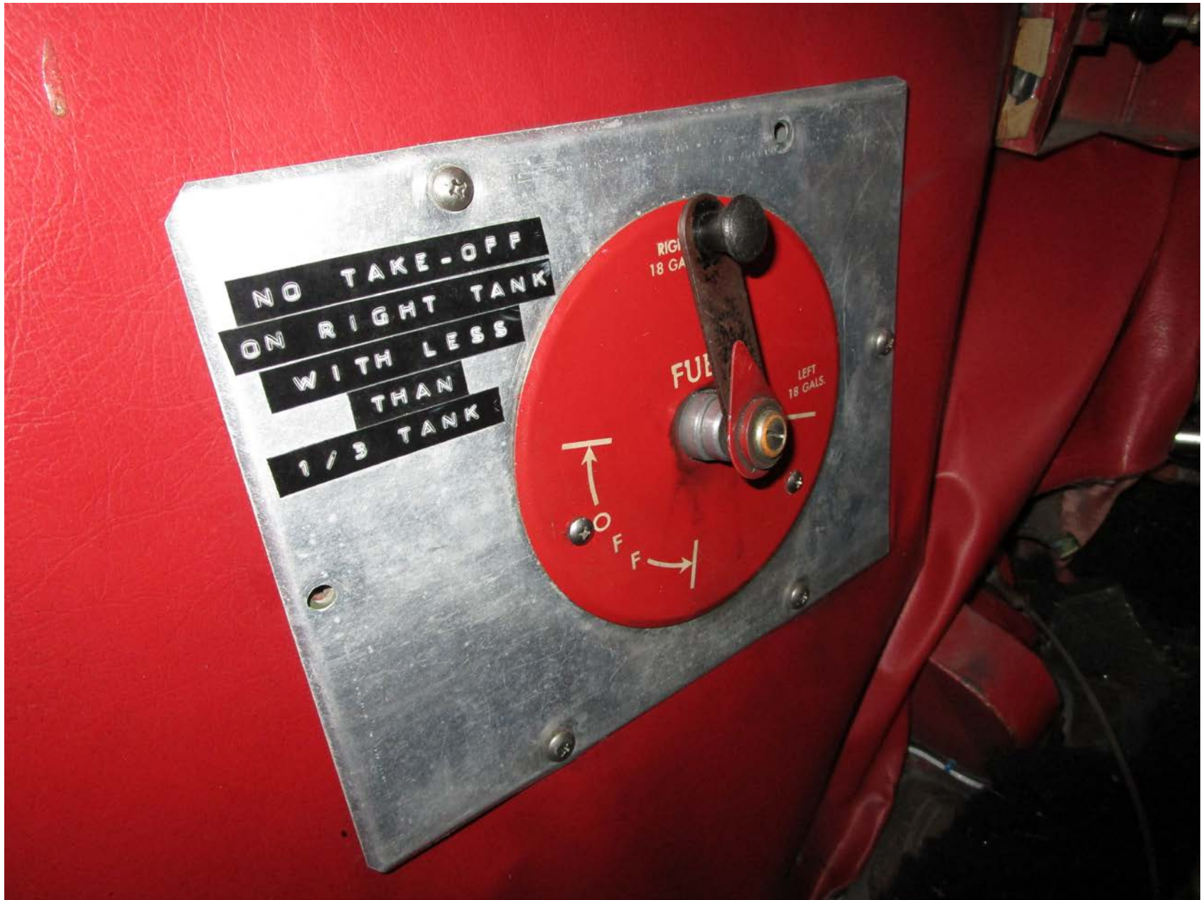
Photo 4 - View of the fuel tank selector valve. (Supplied Photo)
