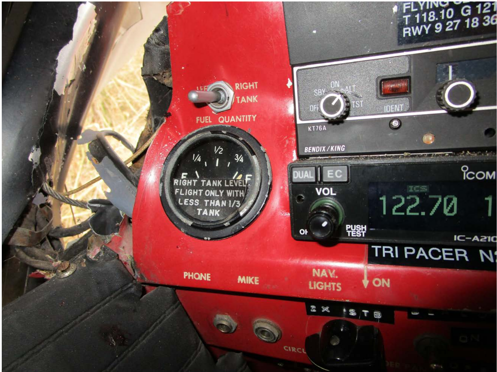
Photo 3 - View of the fuel gauge and fuel tank sender selector switch. (Supplied Photo)
