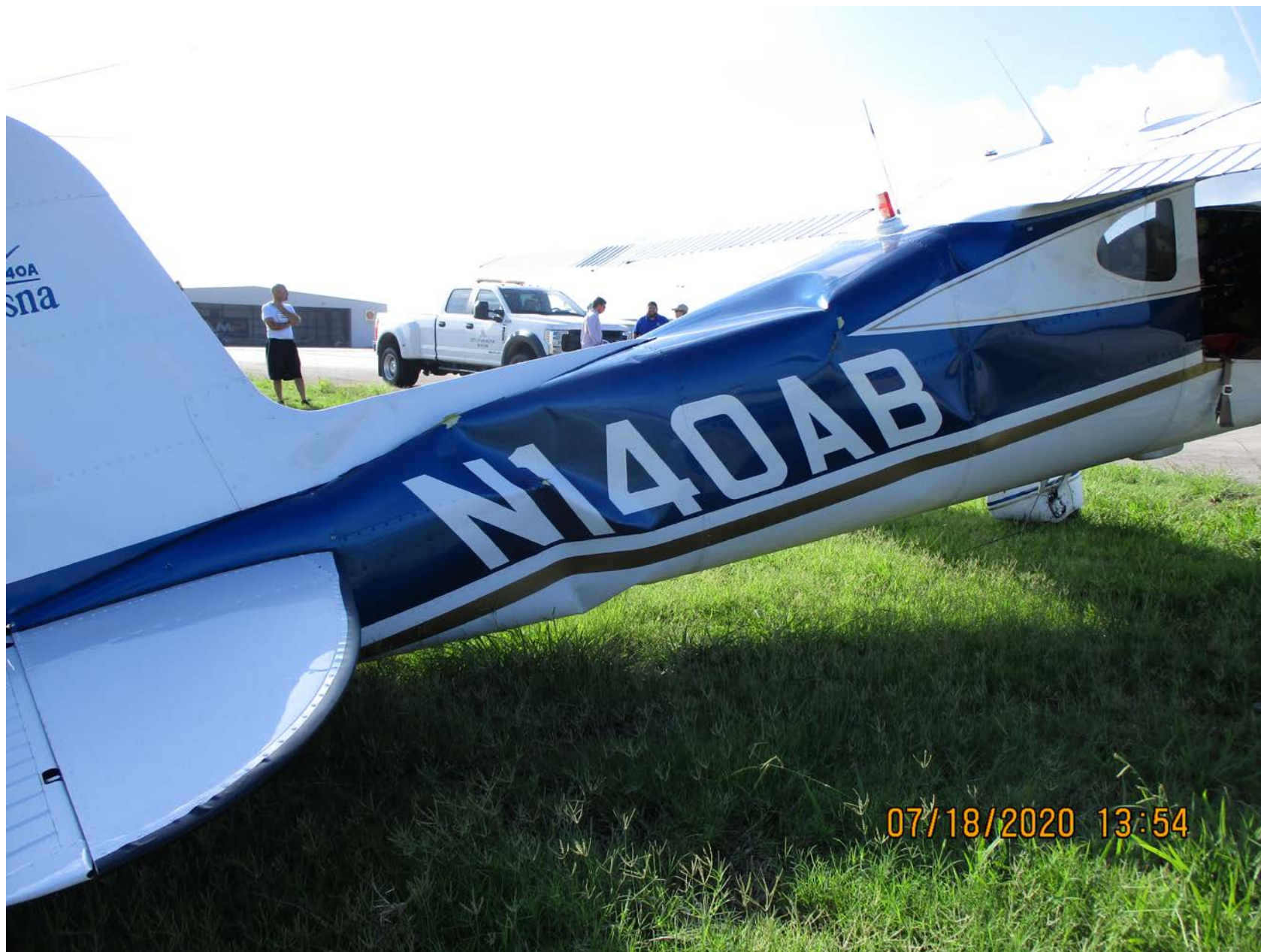
Photo 1 – Supplied image of the right-side fuselage. The fuselage exhibits wrinkle deformation.
