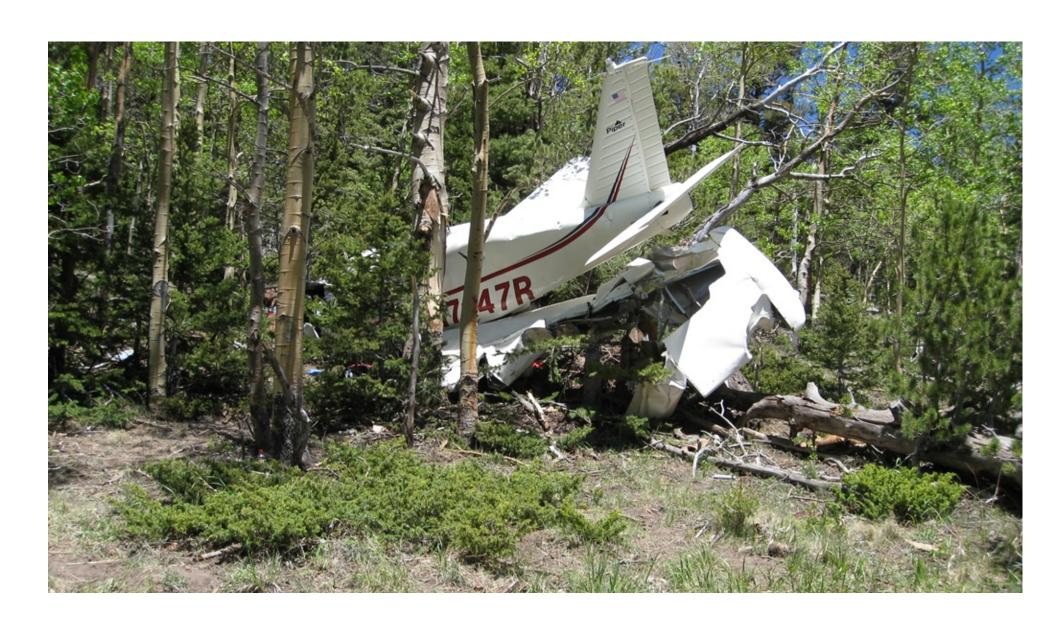
Photo 2 – Accident Site (Aft Fuselage, Left wing, and Empennage)
