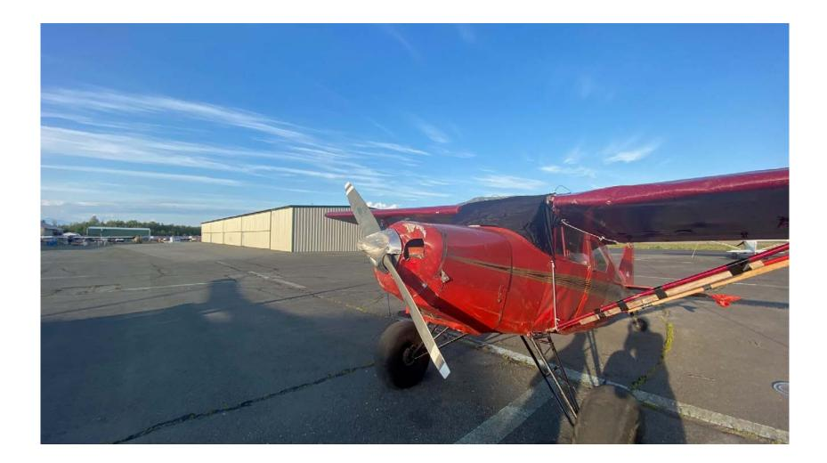
Photo 1 – N7208D PA-22 after recovery exhibiting damage to left wing lift strut and left horizontal stabilizer. (Photograph courtesy of airplane owner.)
