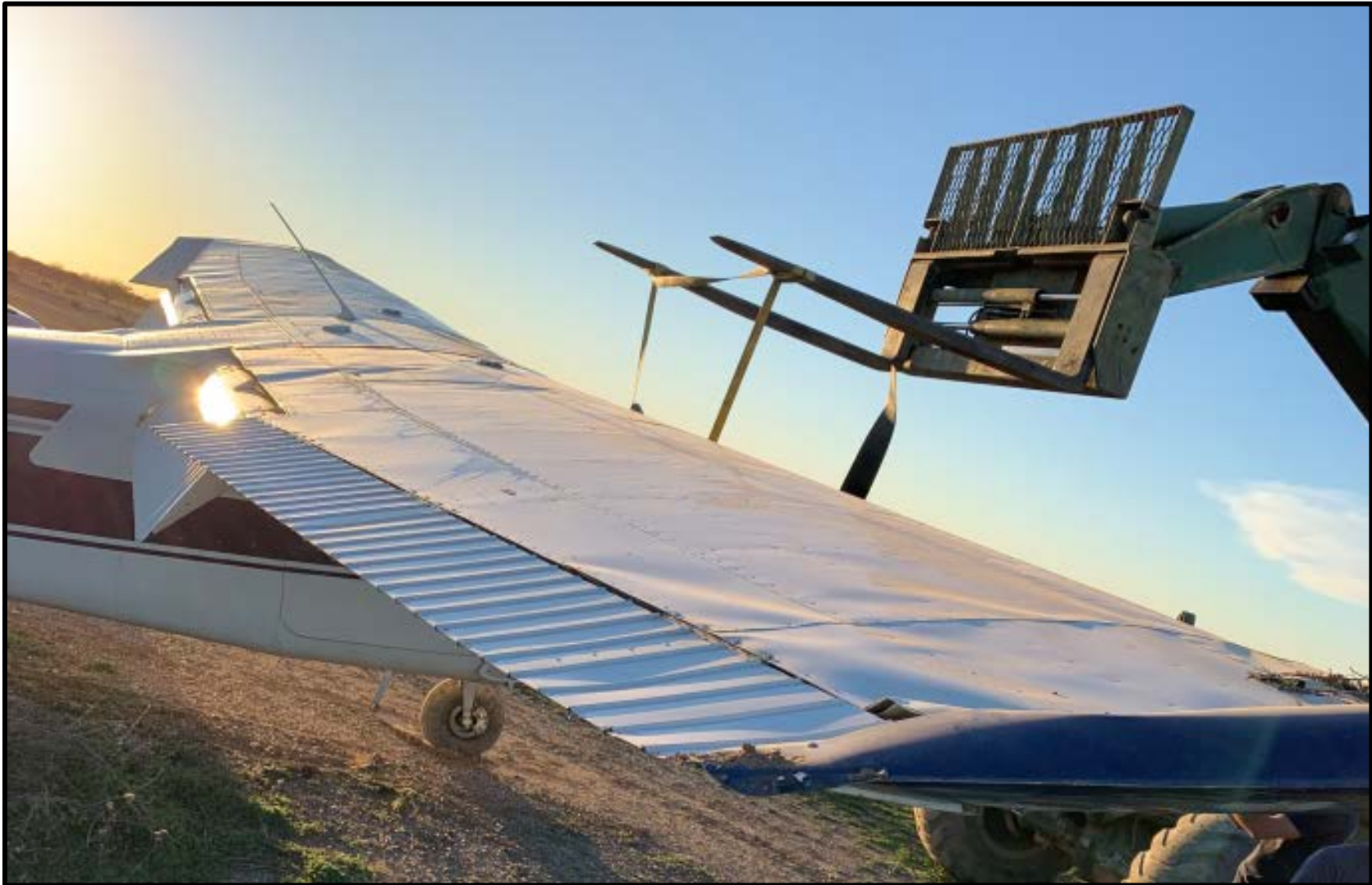
Figure 1: Airplane Damage: Wings
