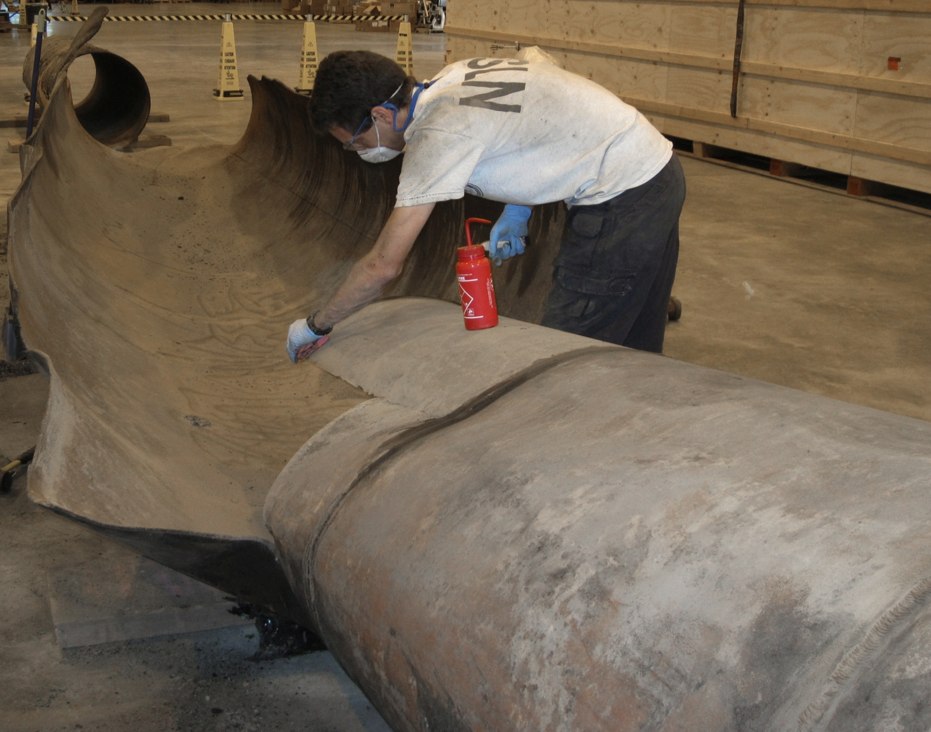
Photograph showing a view of the ruptured pipe piece with an NTSB investigator examining the fracture surfaces
