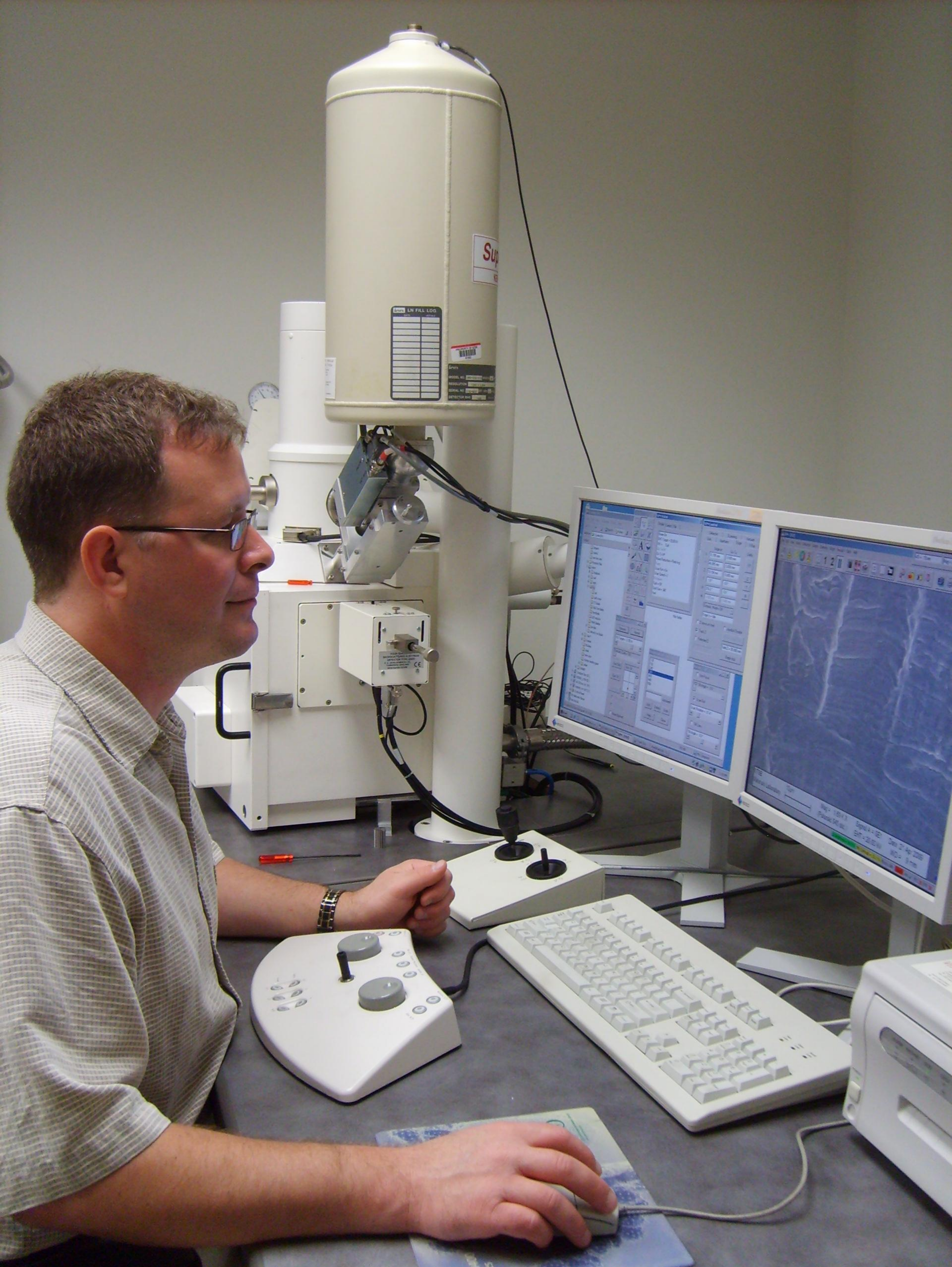
Photograph of an NTSB investigator examining a fracture surface on a scanning electron microscope
