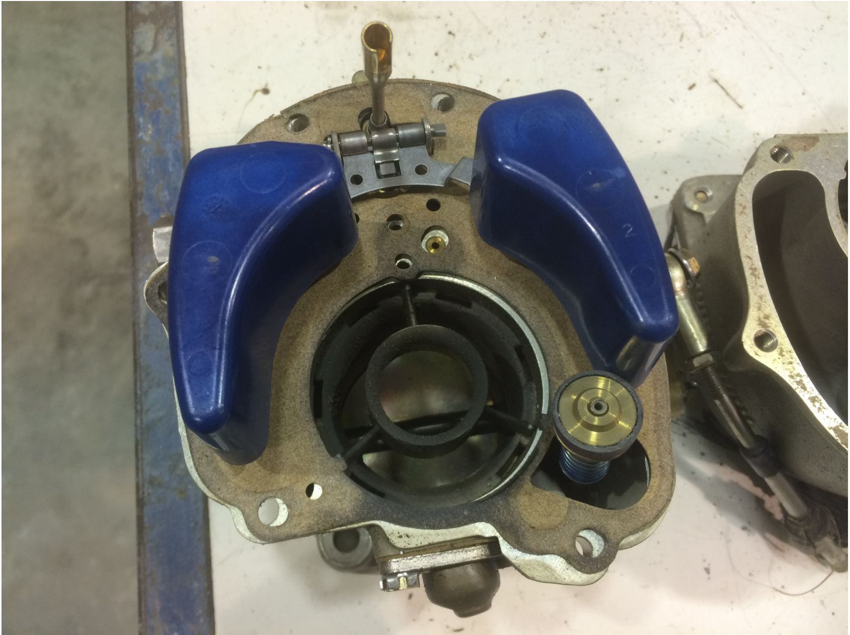
Photo 10 – Carburetor upper half
