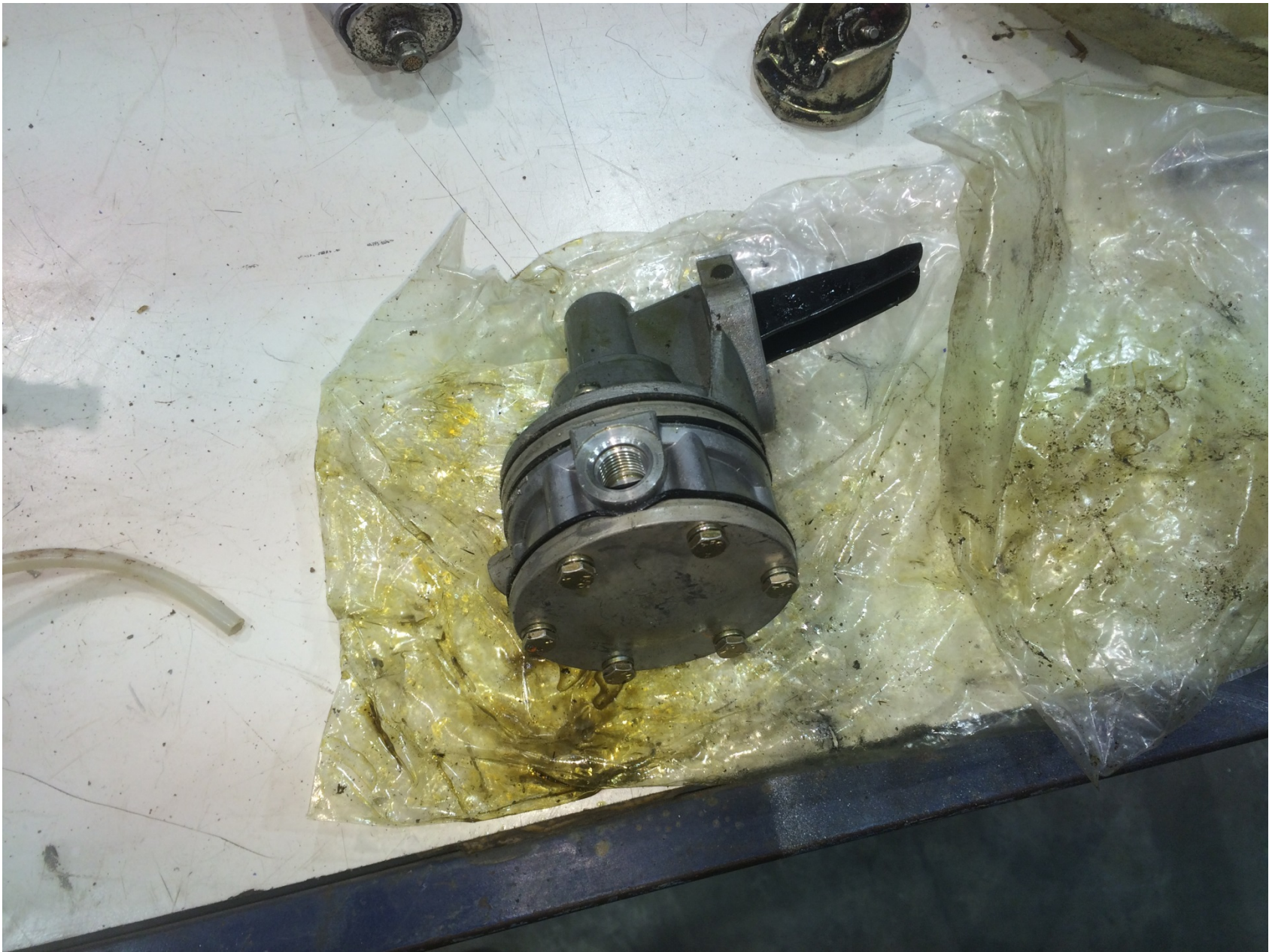
Photo 15 – Mechanical fuel pump found in plastic bag
