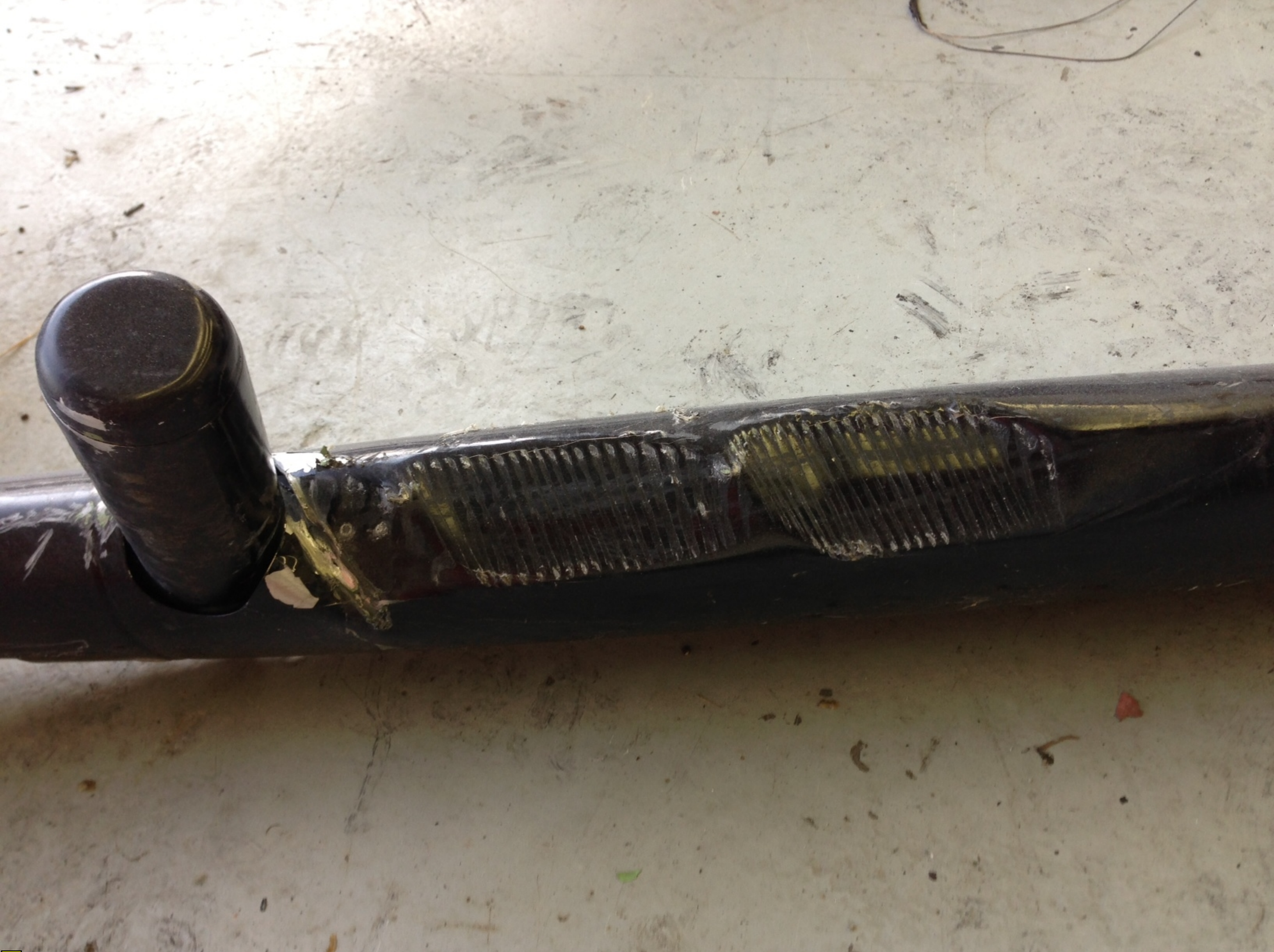
Photograph # 9 – View of wire strike damage observed on skid strut
