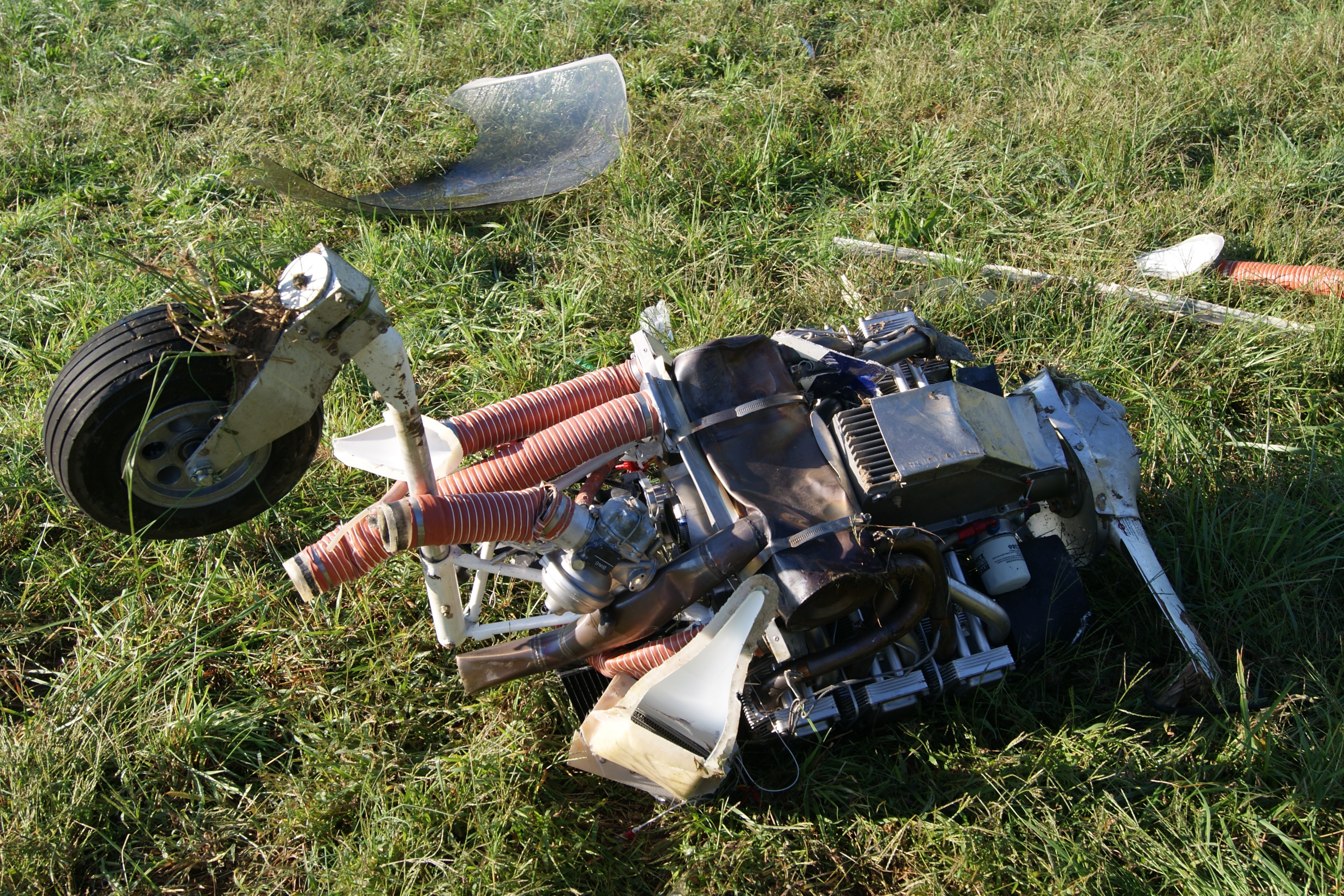
Photograph # 9 - Engine as it came to rest with nose gear attached
