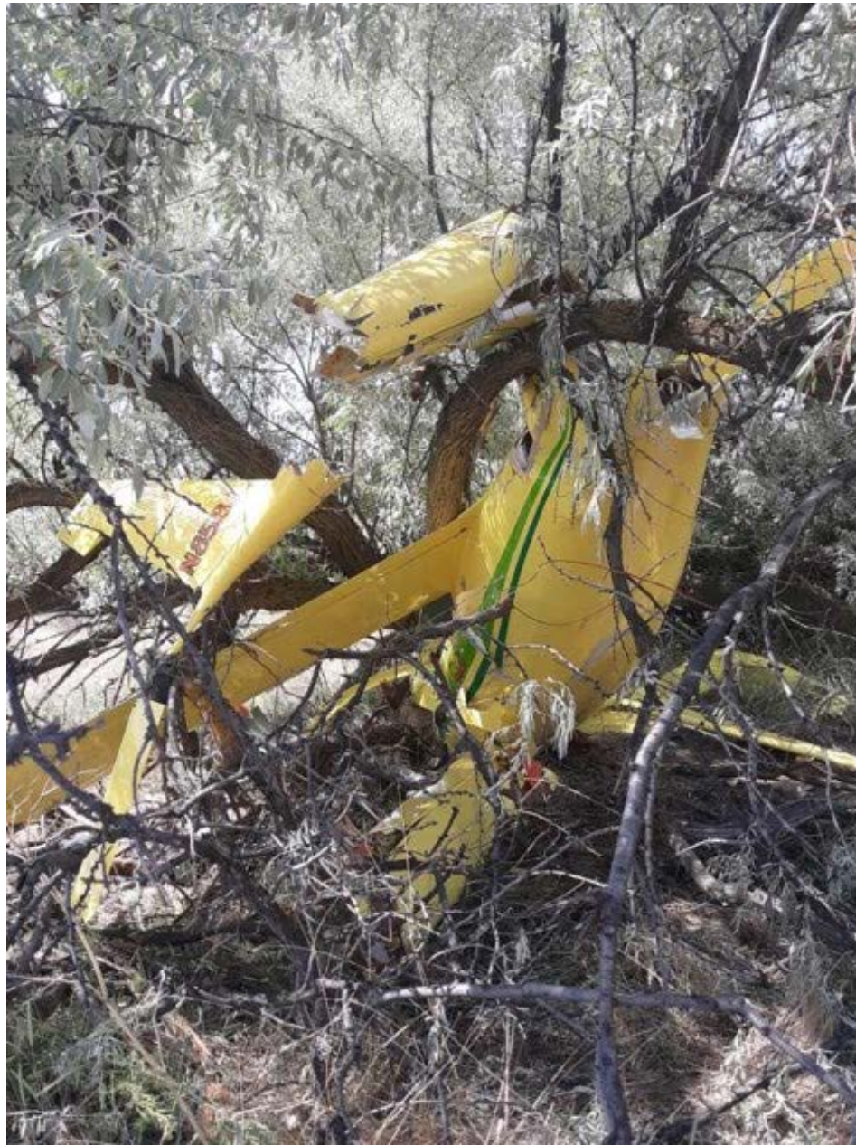
Photo 1 – View of substantial damage to wings, canard and empennage (Courtesy of FAA)
