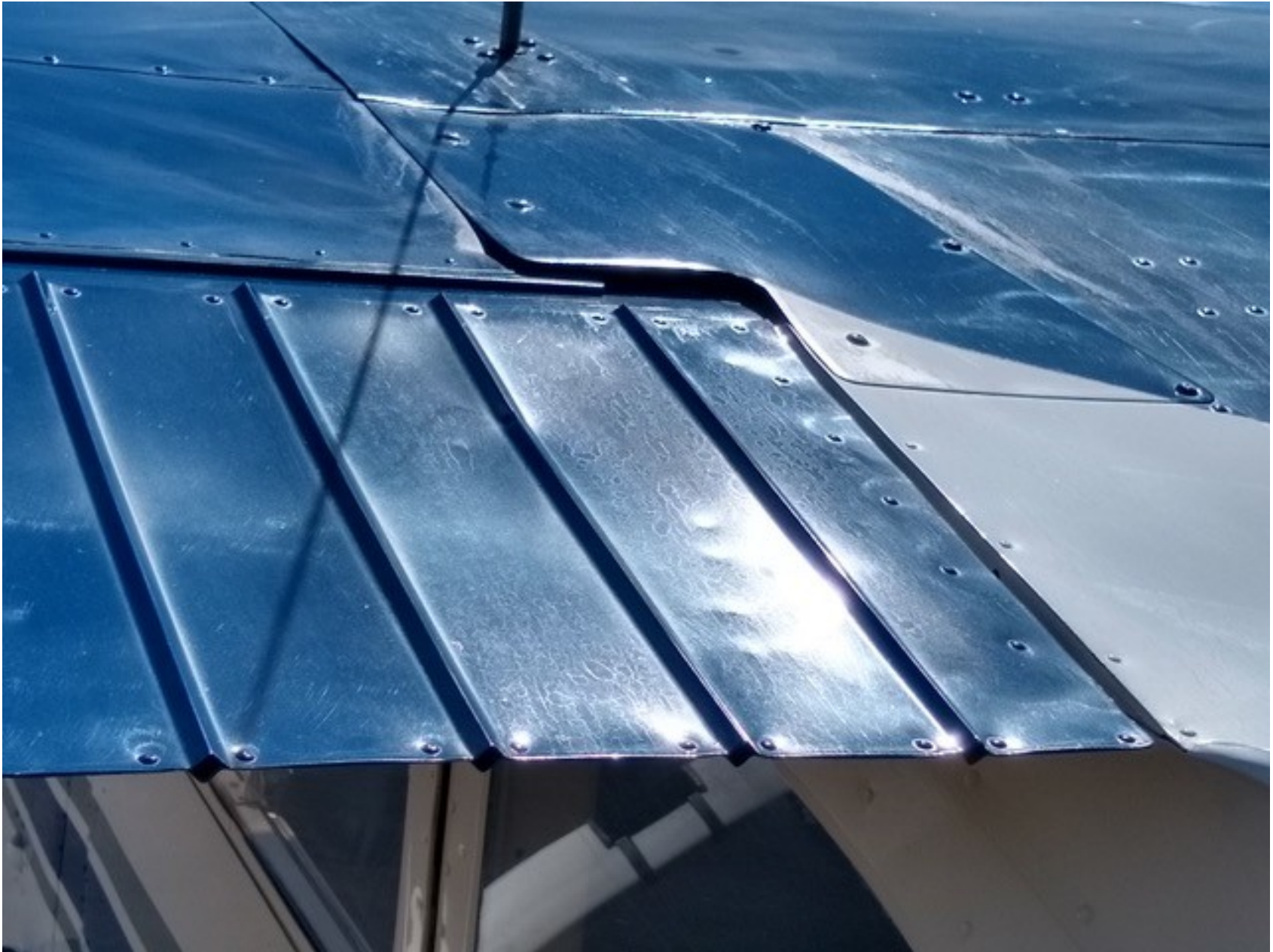
Photo 1 – Substantial damage to the wing root
