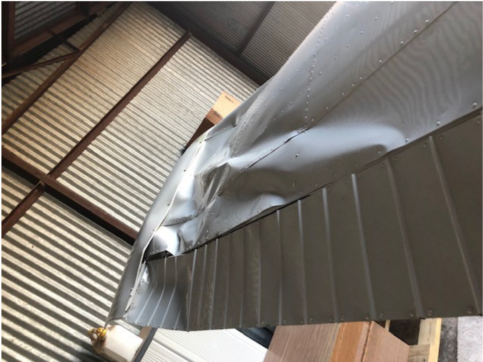
Photo 1 – View of damage to the left wing and aileron (Courtesy of FAA)
