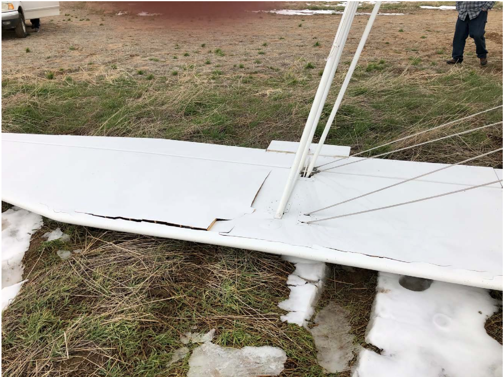
Photo 1 – View of damage to the upper left wing (Courtesy of FAA)
