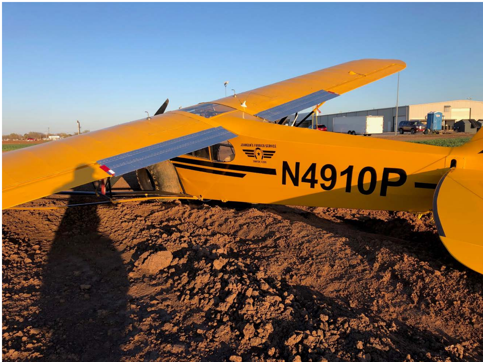
Photo 1 – View of damage to the left wing lift struts (Courtesy of Operator)
