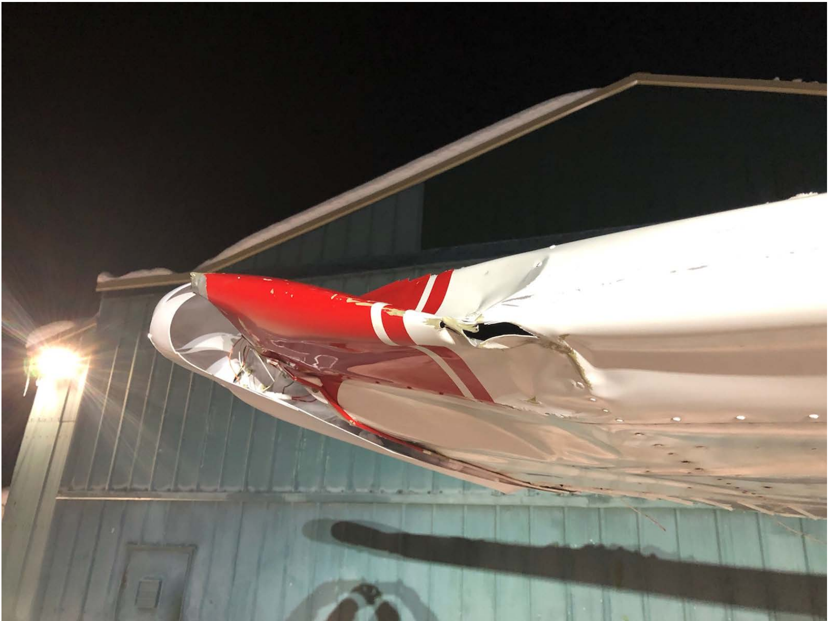
Photo 1 – Accident airplane's damaged right wing.
