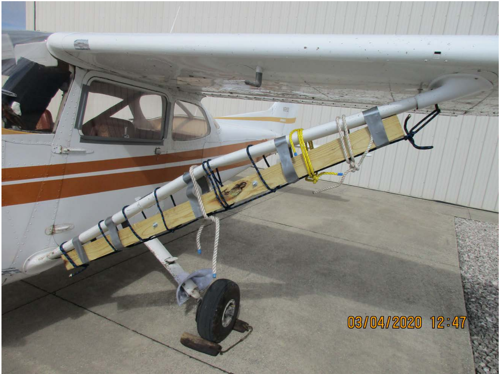
Photo 1 – View of damage to the left wing lift strut (Courtesy of FAA)
