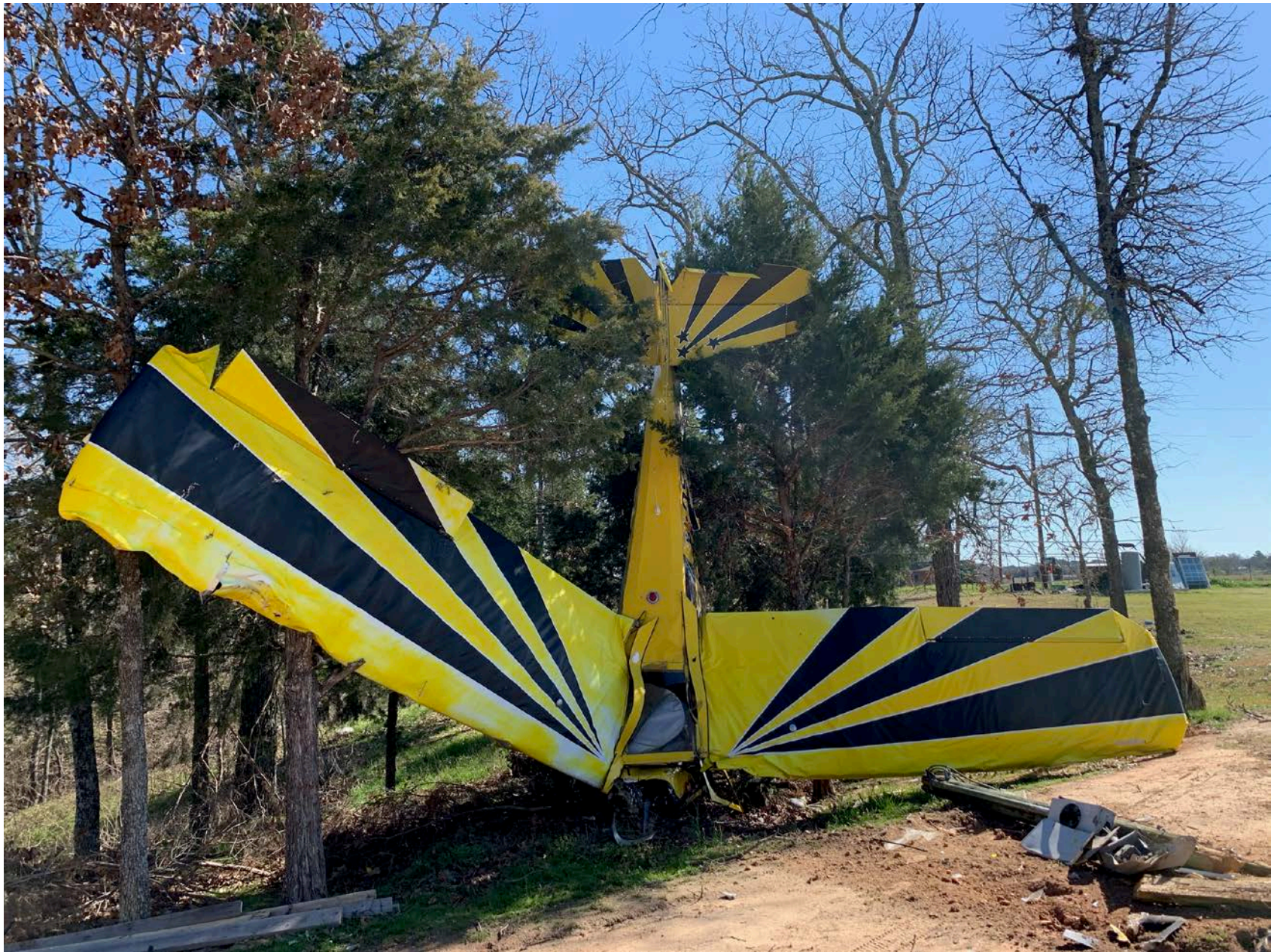
Photo 1 – View of damage to both wings (Courtesy of Operator)
