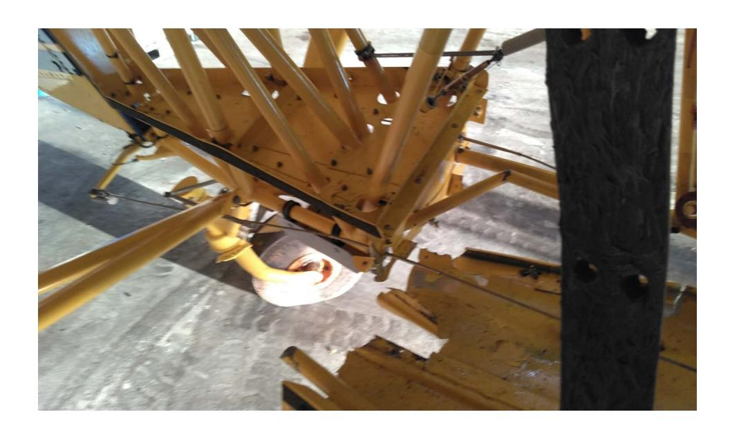
Photo 1 – View of damage to the airplane's longerons (Courtesy of Operator)
