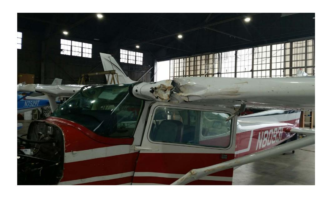
Photo 1-View of damage to both wings and the left wing lift strut (Courtesy of FAA)
