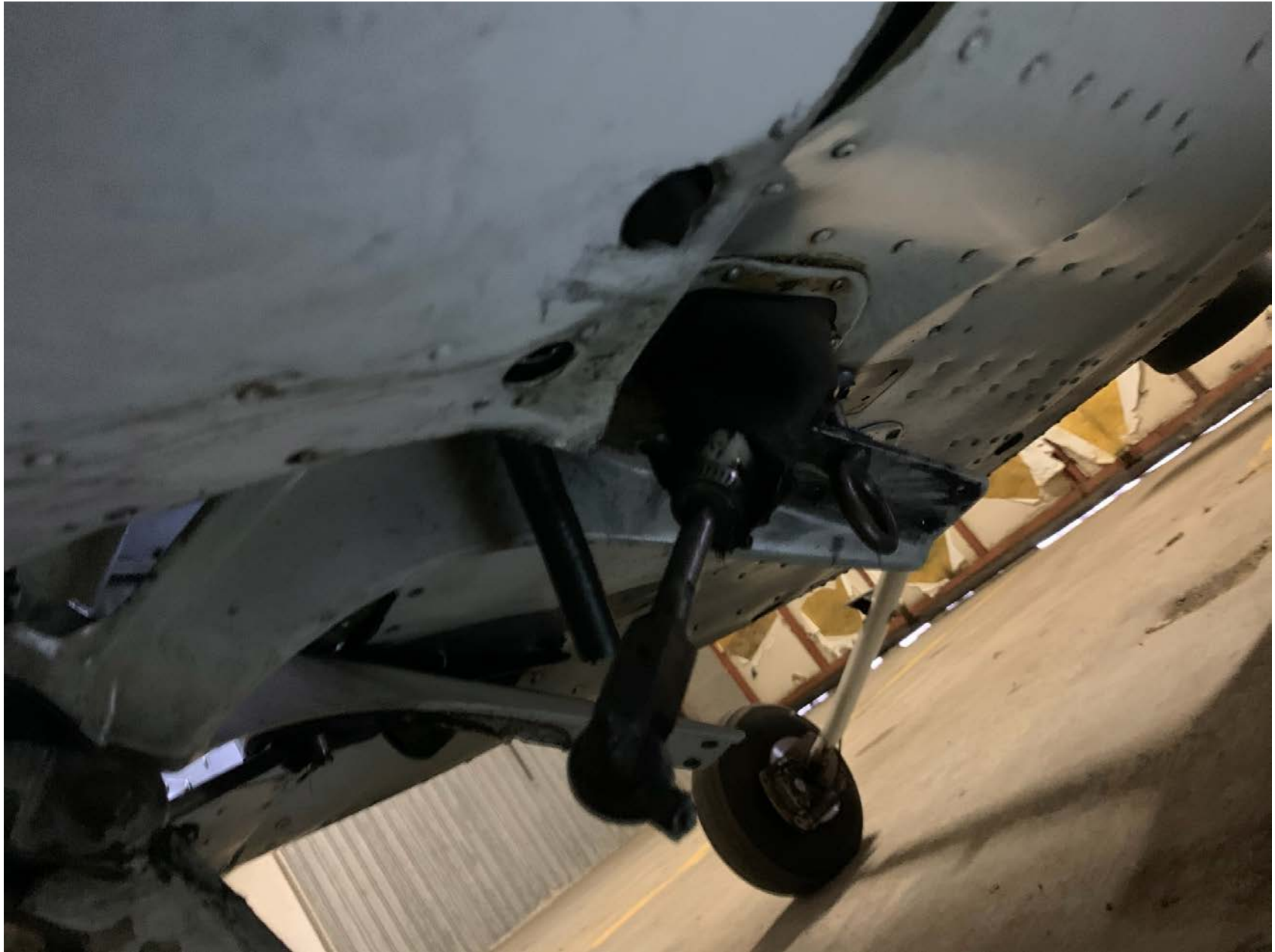
Photo 1 – View of lower fuselage damage (Courtesy of FAA)
