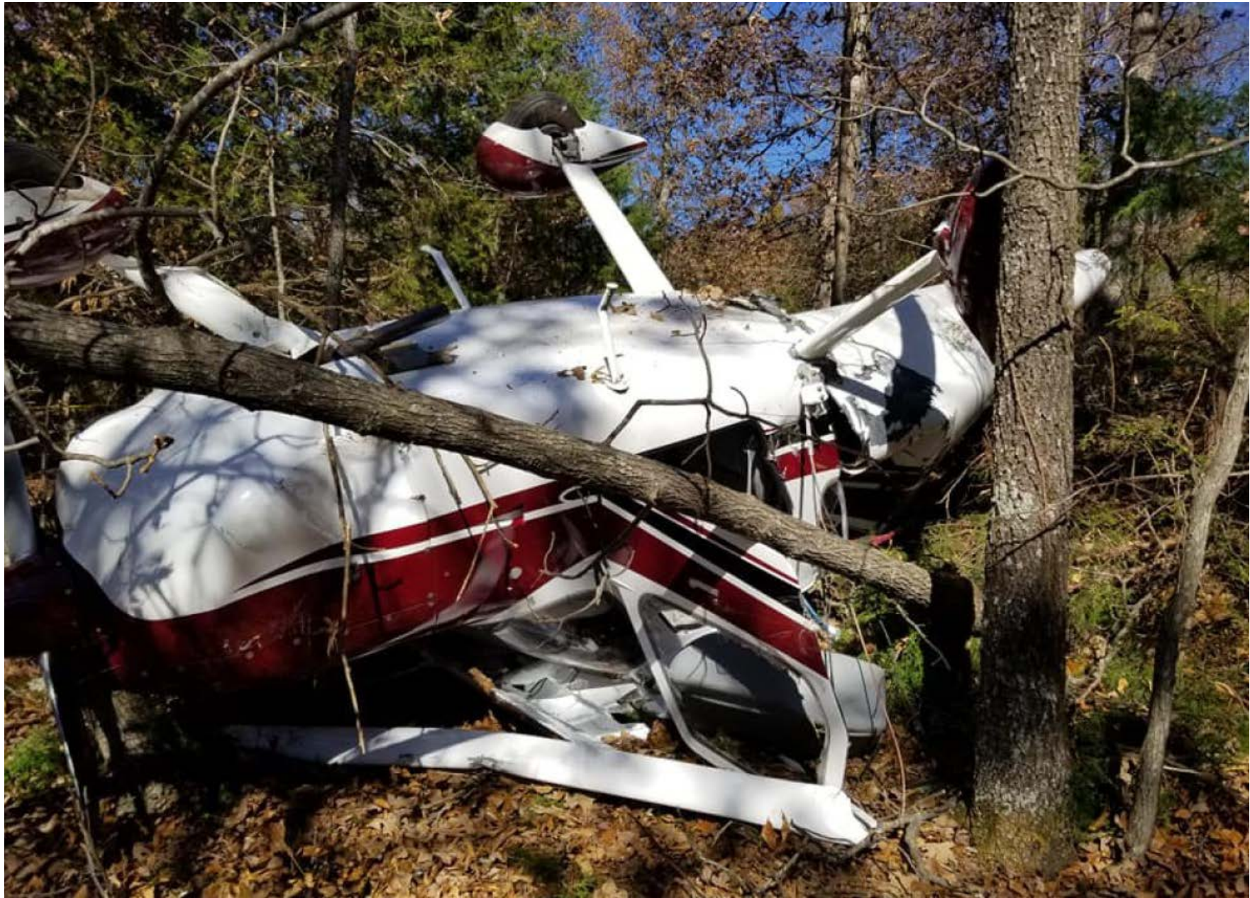
Photo 1 – View of substantial damage to the right wing and fuselage (Courtesy of FAA)
