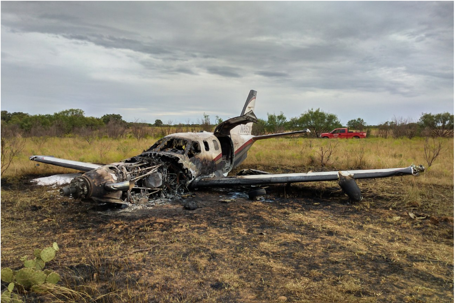
Photo 1 – View of the substantial damage to the airplane’s windscreen (Courtesy of FAA)
