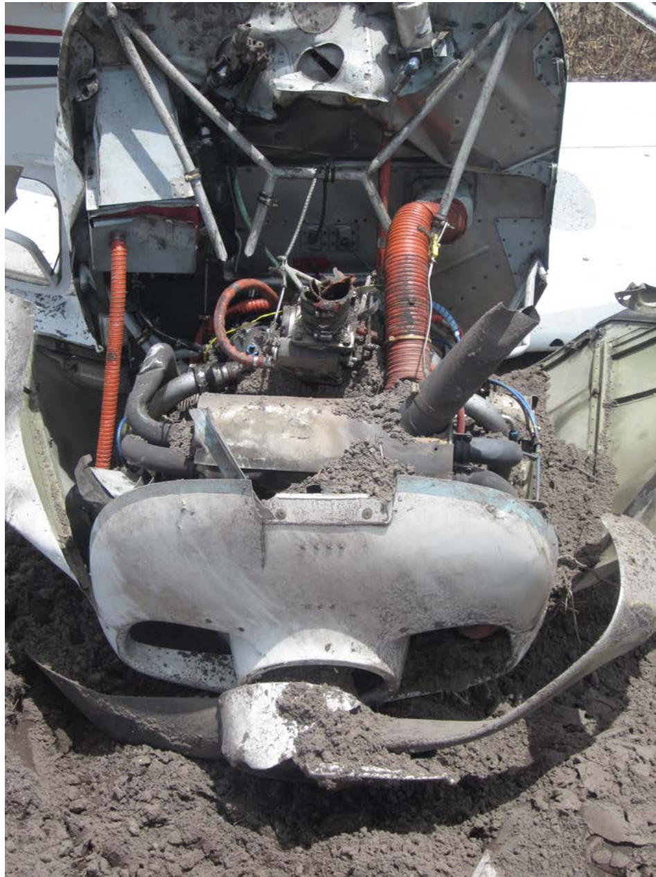
Photo 1 – View of damage to the engine mounts (Courtesy of FAA)
