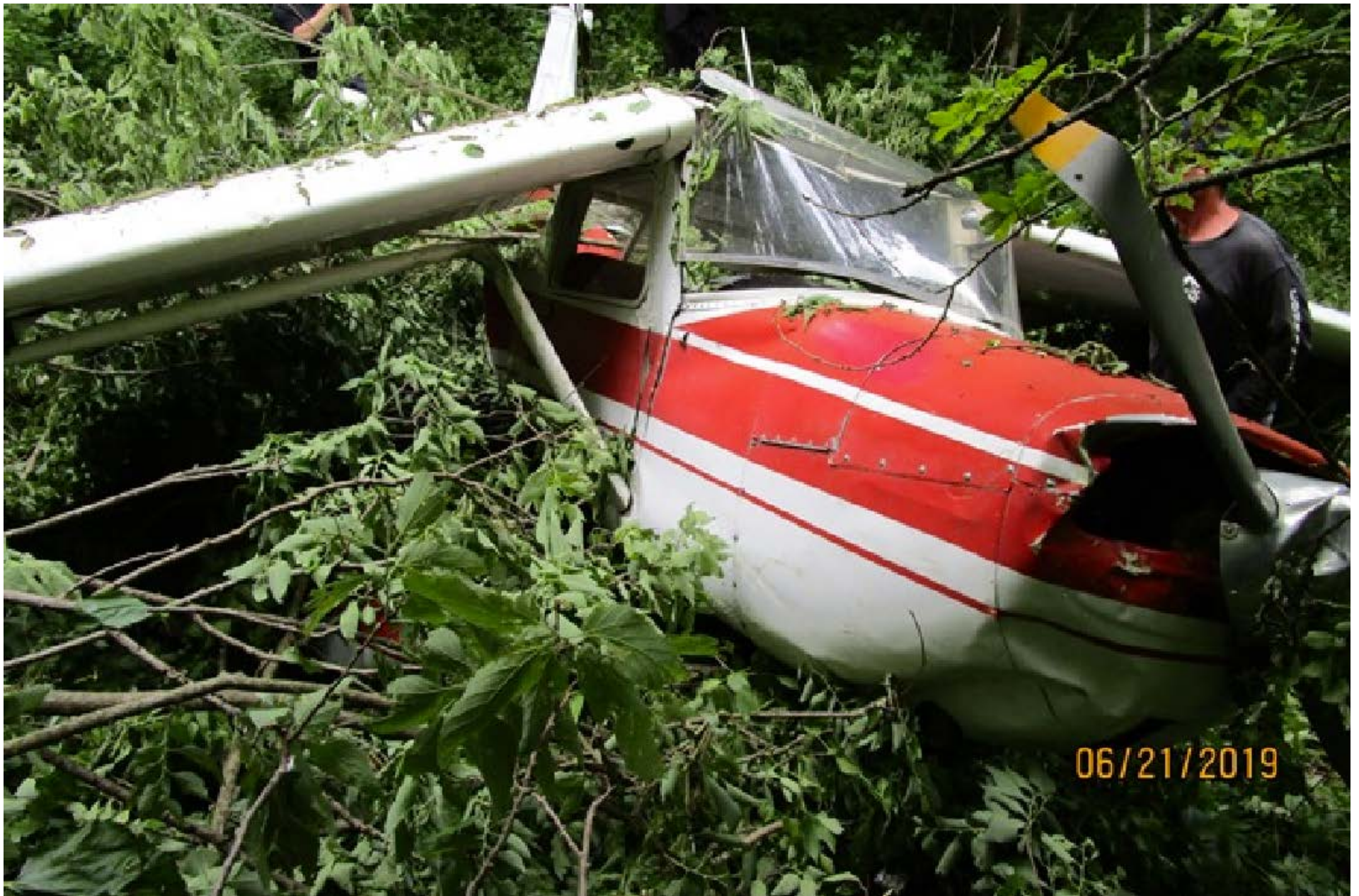
Photo 1 – View of substantial damage to the right wing and the right wing lift strut (Courtesy of FAA)
