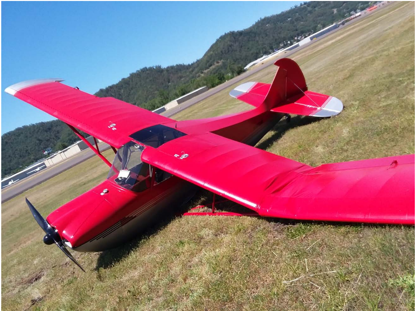
Photo 1 – View of damage to the left wing (Courtesy of FAA)
