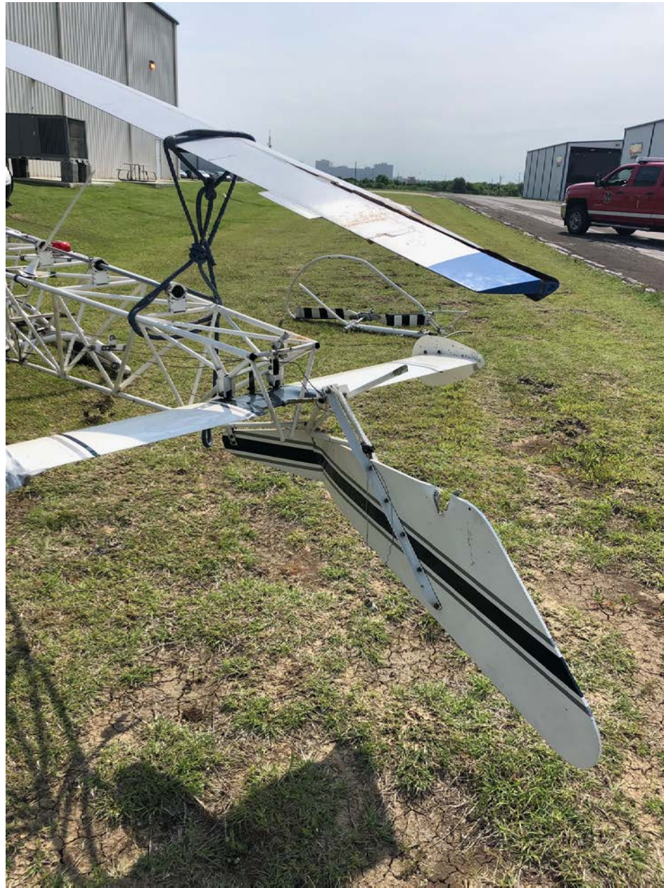
Photo 1 – View of damage to the tailboom and tailrotor drive system (Courtesy of FAA)
