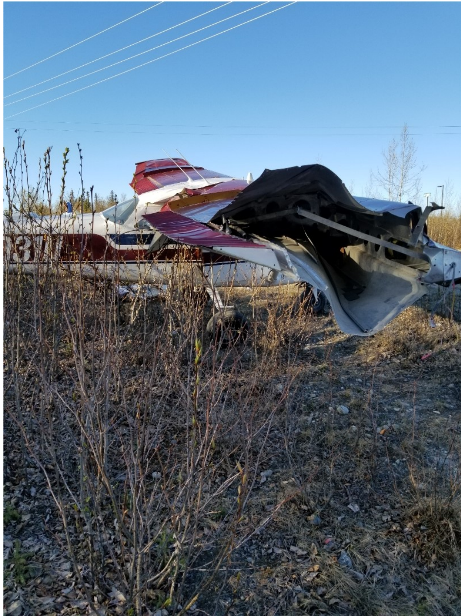
Photo 1 – View of damage to the right wing (Courtesy of FAA)
