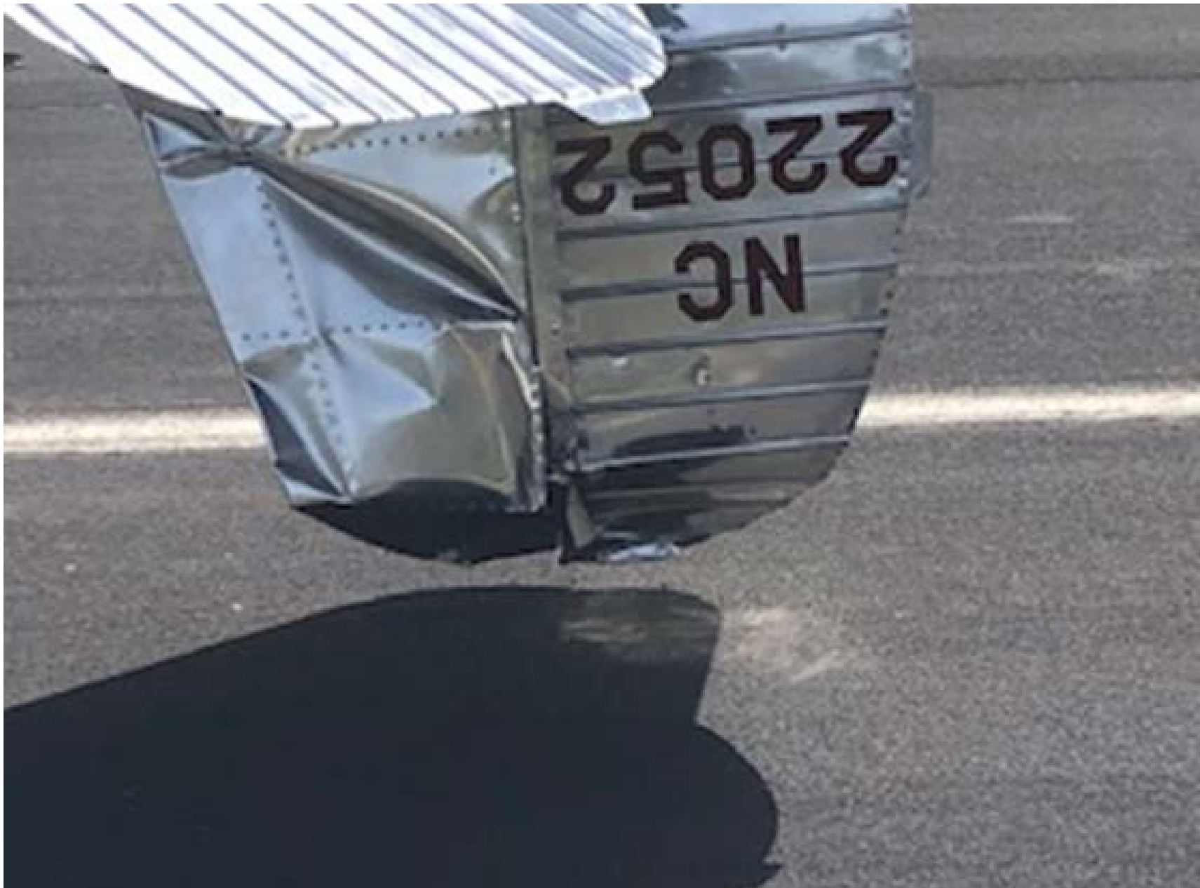
Photo 1 – View of damage to the rudder and the vertical stabilizer (Courtesy of FAA)
