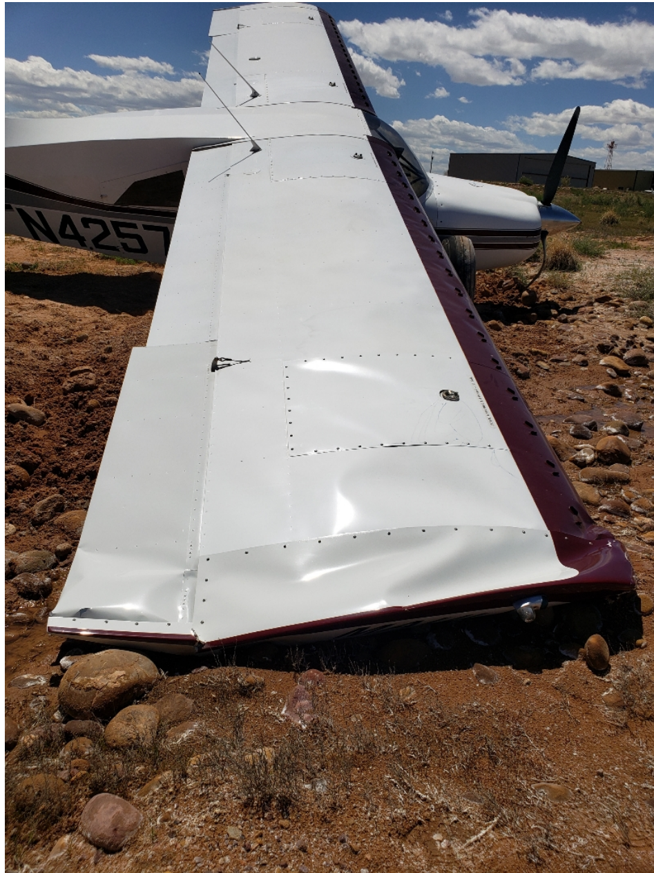
Photo 1 – View of damage to the right aileron (Courtesy of FAA)
