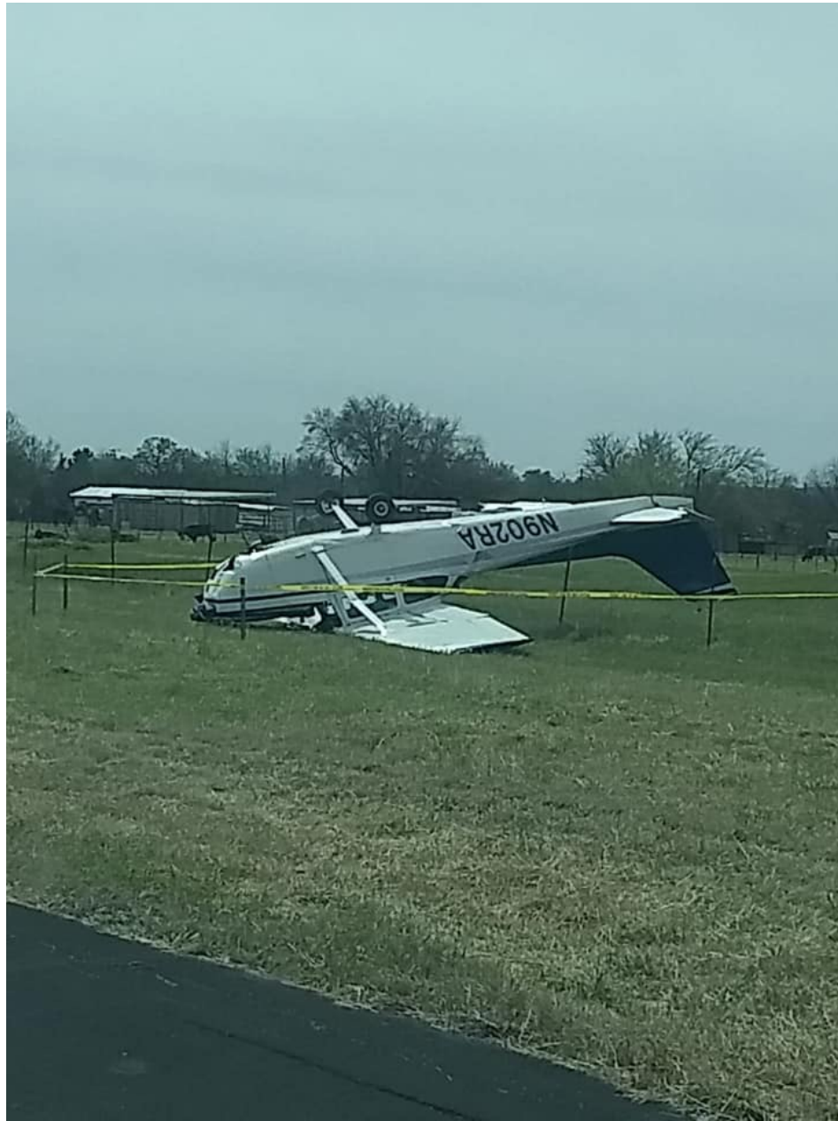
Photo 1 – View of damage to the right wing lift strut (Courtesy of FAA)
