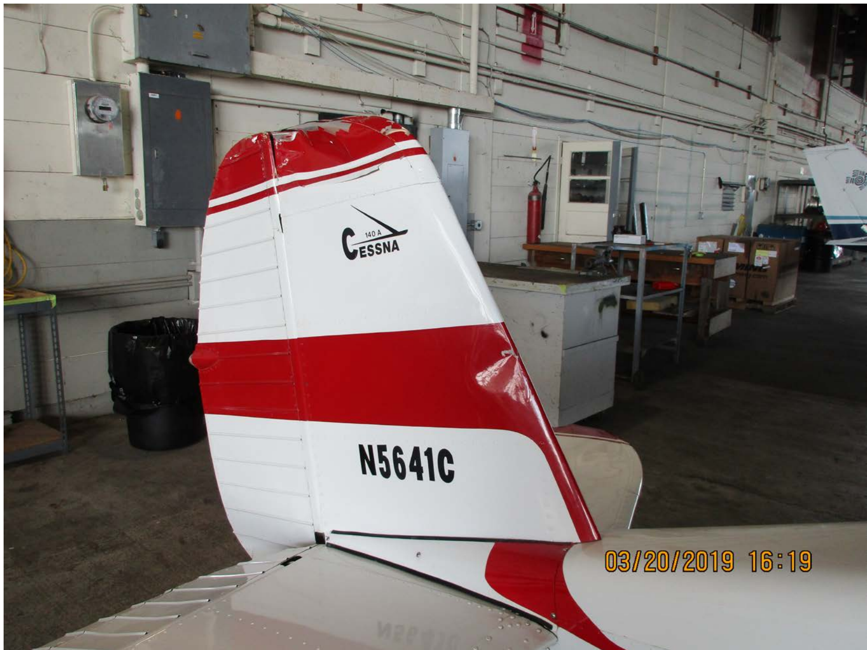
Photo 1 – View of damage to the rudder and horizontal stabilizer (Courtesy of FAA)
