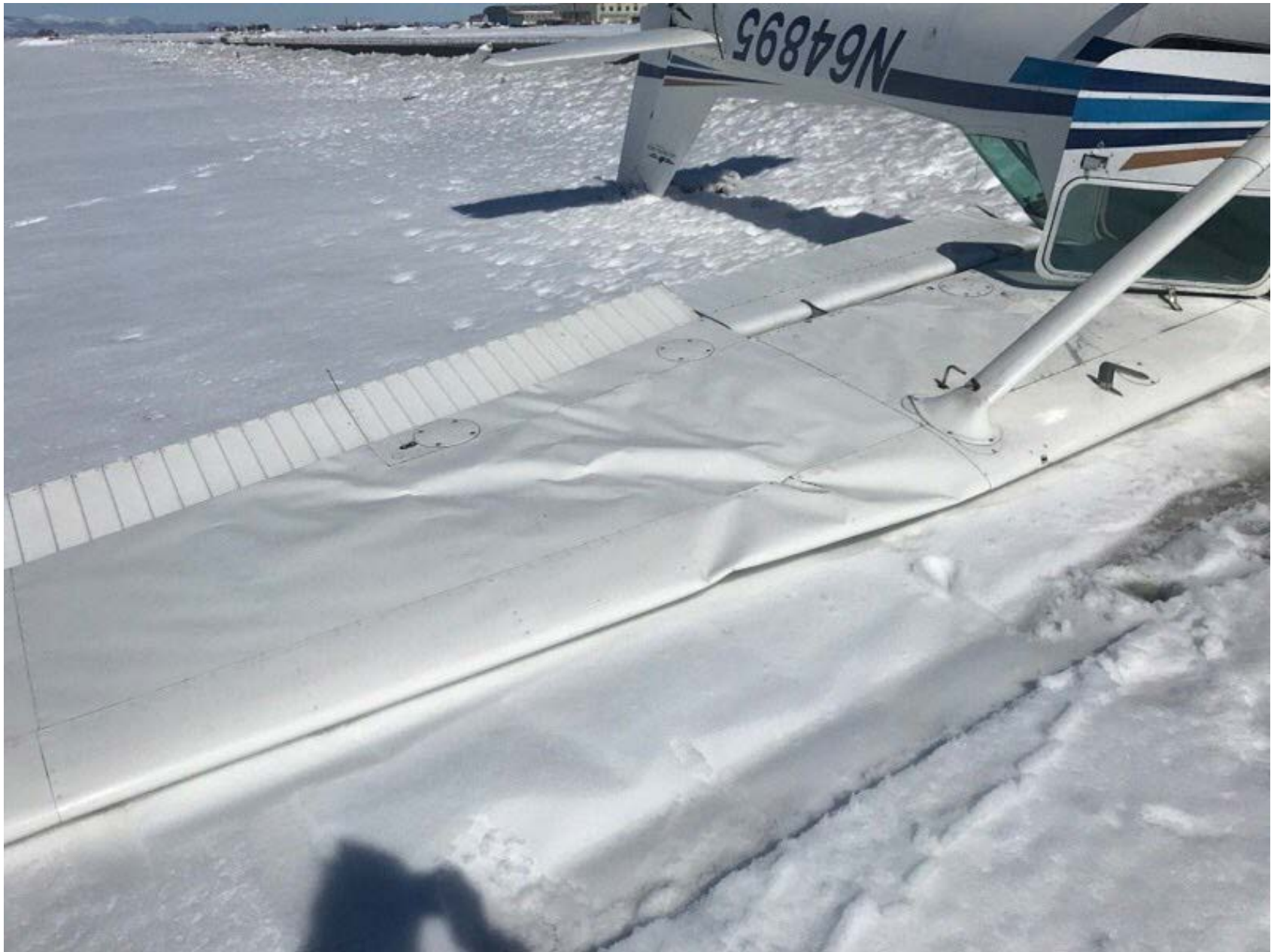
Photo 1 – View of damage to the airplane’s left wing (Courtesy of FAA)
