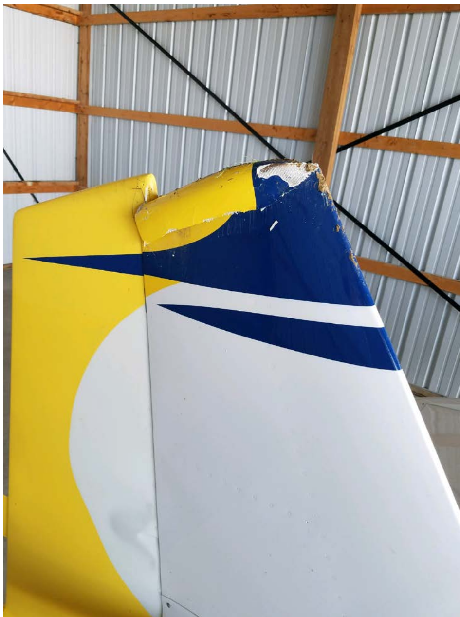
Photo 1 – View of damage to the rudder and vertical stabilizer (Courtesy of FAA)
