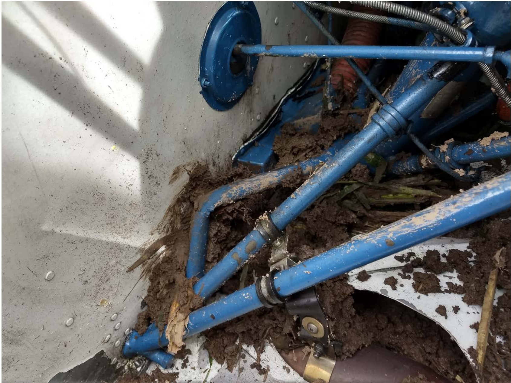
Photo 1 – View of damage to engine mounts (Courtesy of FAA)
