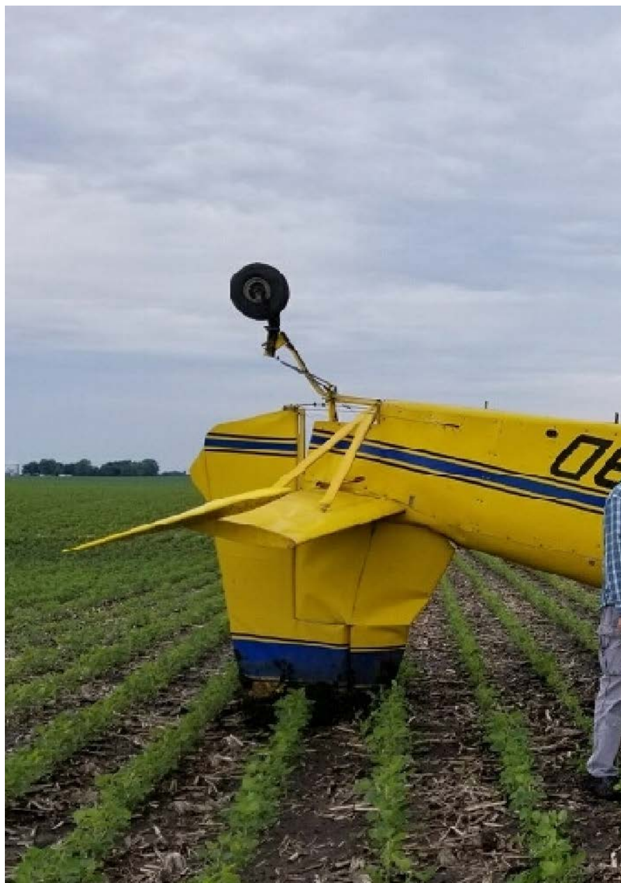
Photo 1 – View of damage to the vertical stabilizer and the rudder (Courtesy of FAA)
