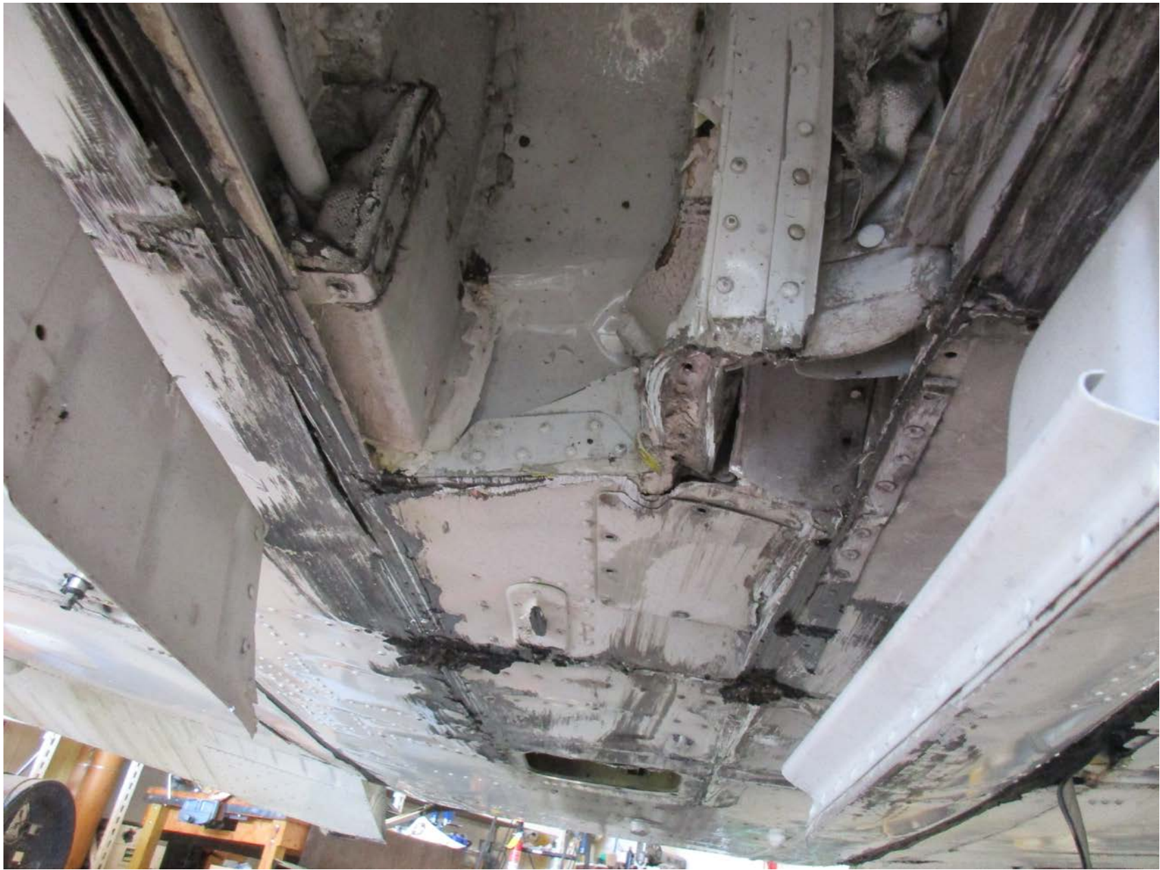
Photo 1 – View of damage to stringers, longerons, and carry through (Courtesy of FAA)
