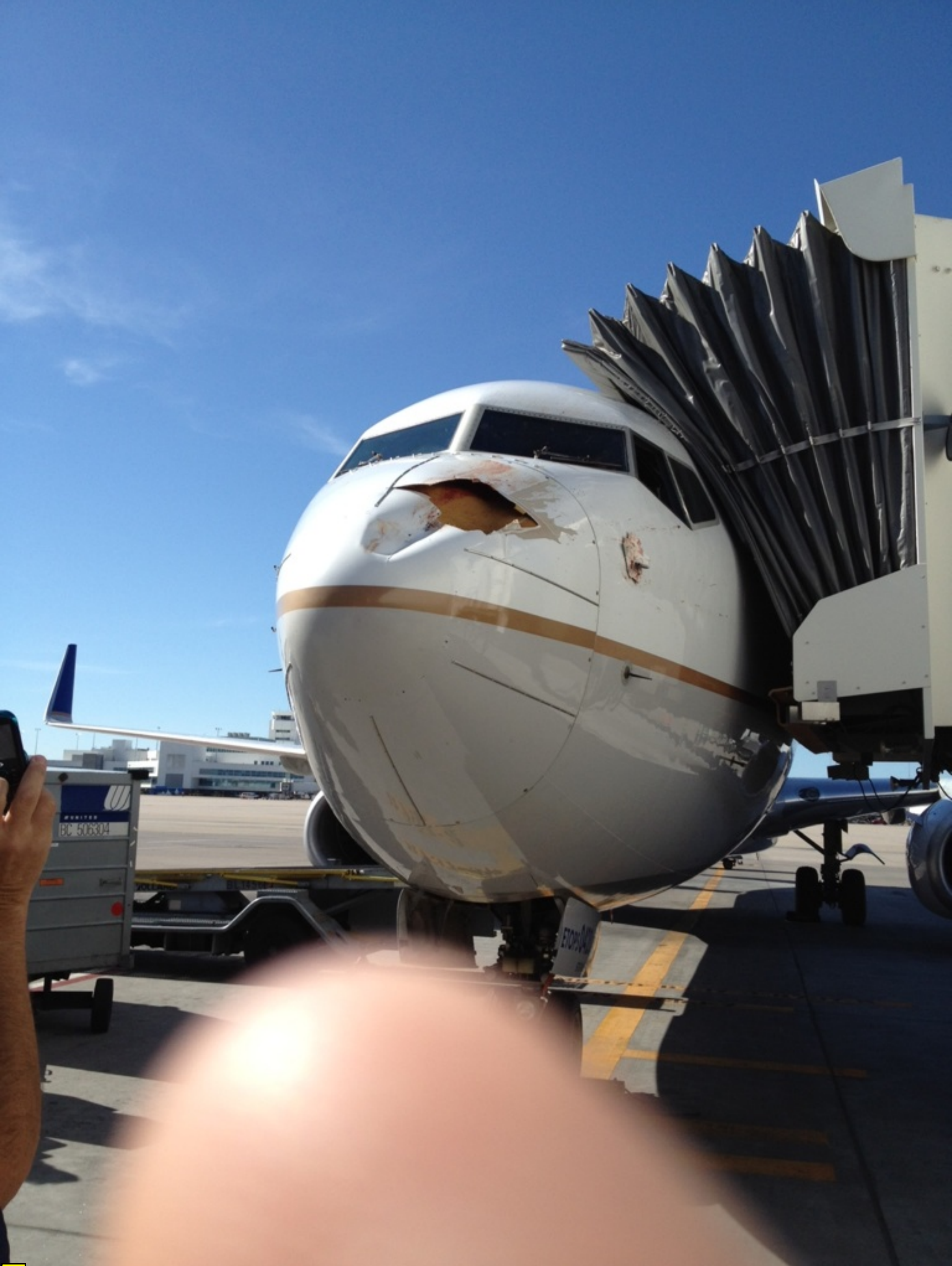
Photo of damage to radome
