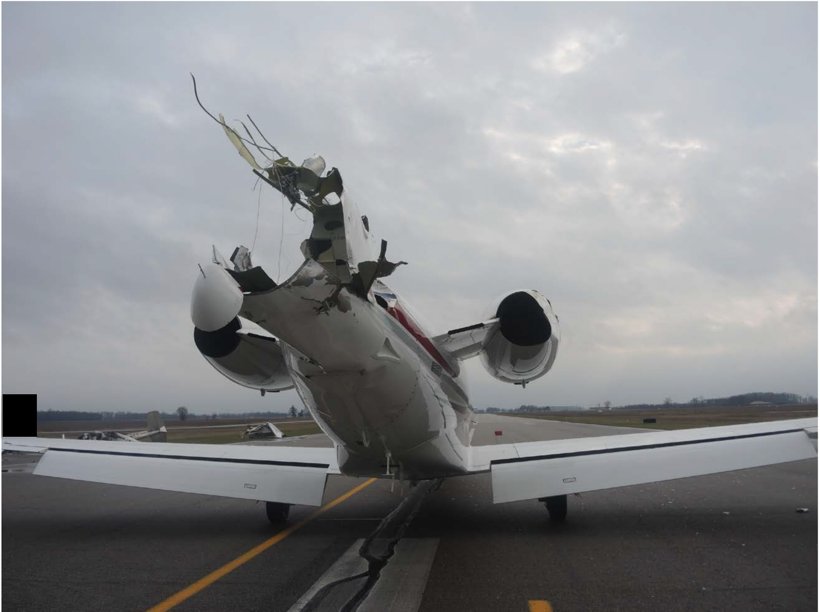
Photo 4 - Accident Site Cessna 525 Empennage Damage
