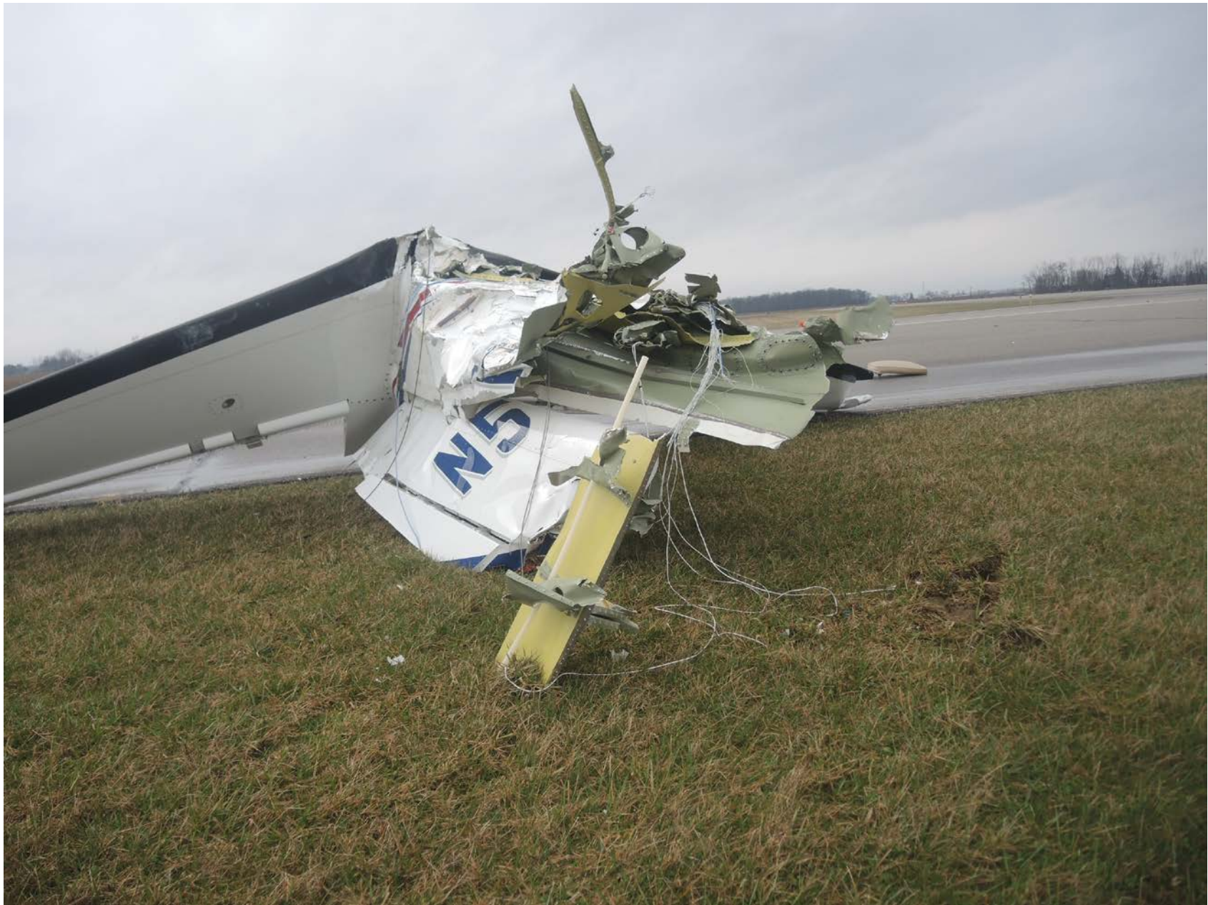
Photo 5 – Accident Site Cessna 525 Separated Empennage
