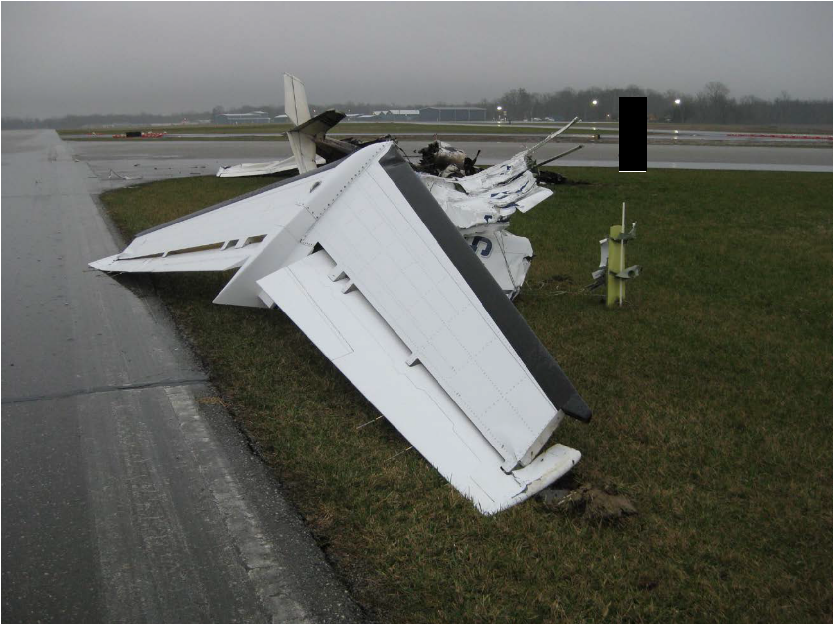
Photo 3 – Accident Site Cessna 150 and Cessna 525 Separated Empennage
