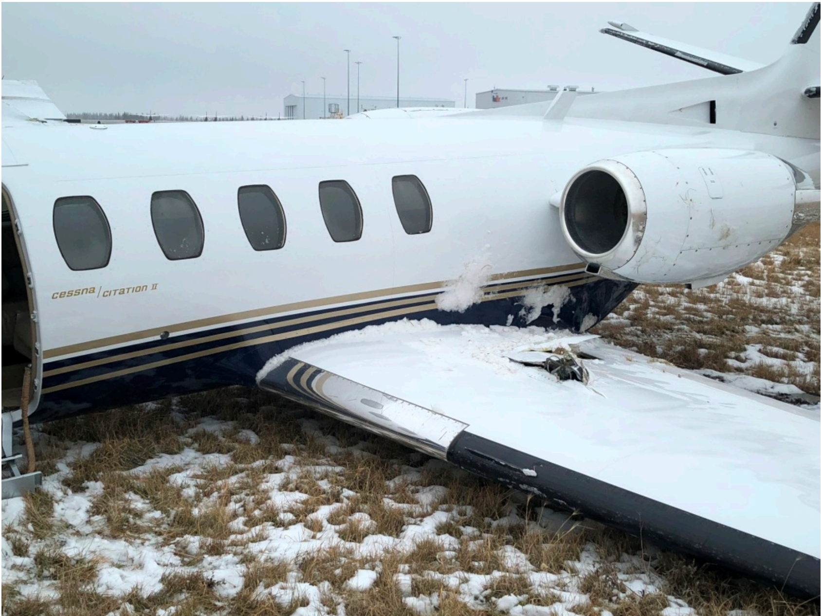
Photo 8 - View of the damage to the left wing (Jet Center photo)
