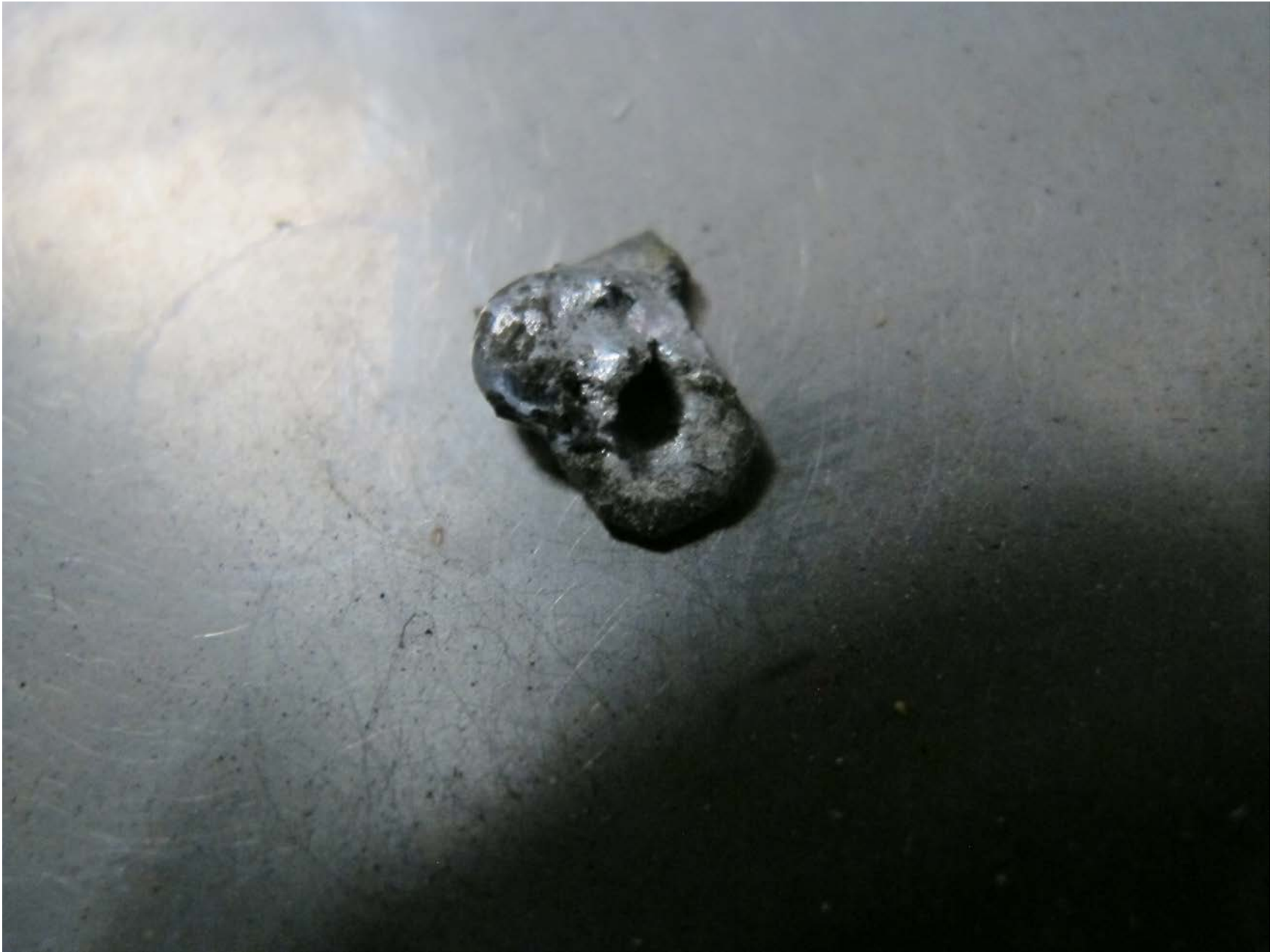
Photo 16 – View of the backside of the terminal fuse holder (RH Photo)
