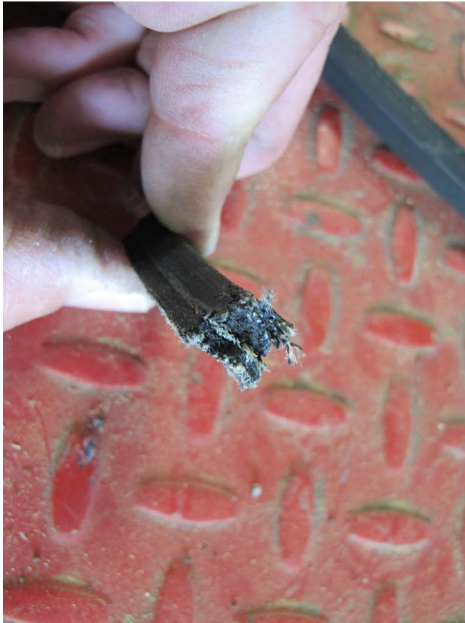
Photo 9 – Fracture surface of small section of V-belt (RH Photo)
