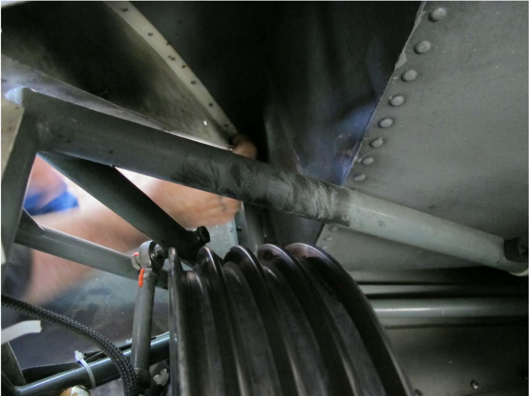
Photo 10 – Rubber residue on frame tube adjacent to V-belt grooves and forward of grooves (RH Photo)
