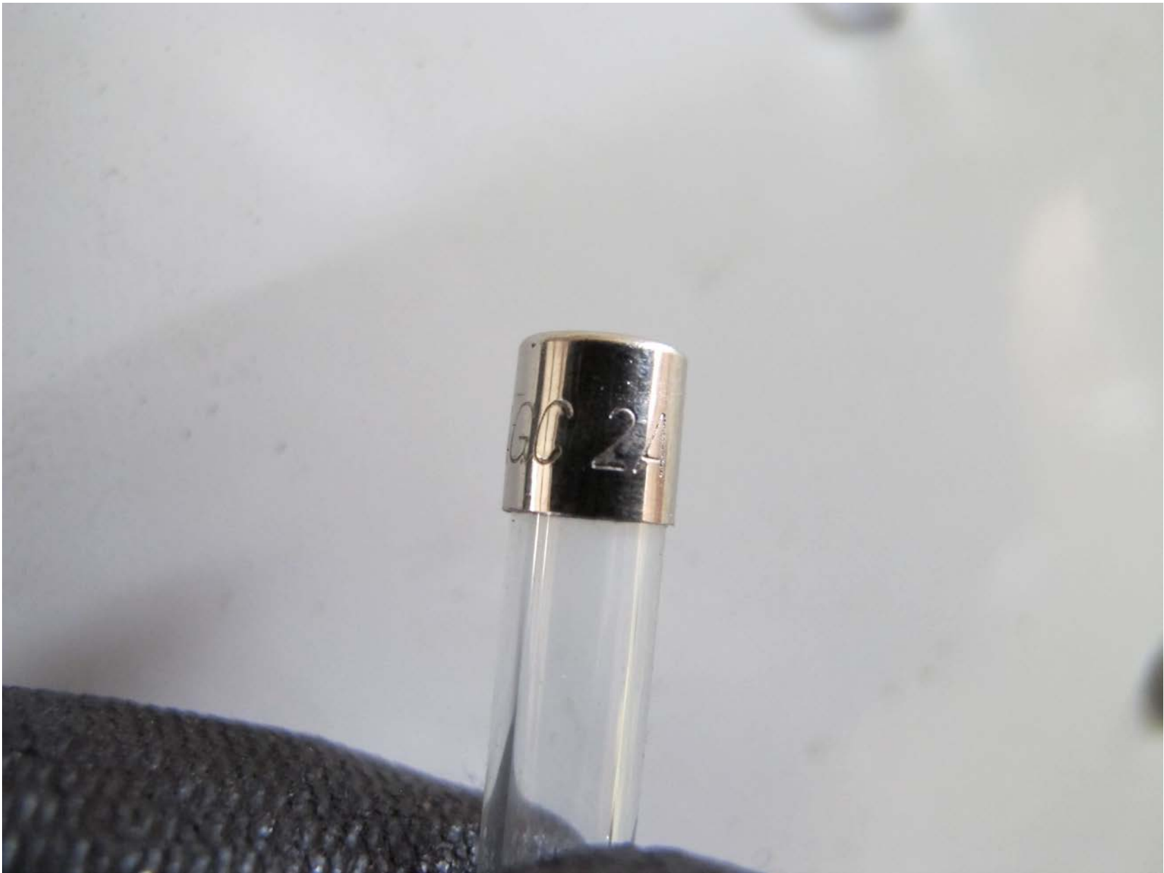
Photo 17 – View of the 2-Amp fuse removed from the fuse holder (Blown) (H Photo)
