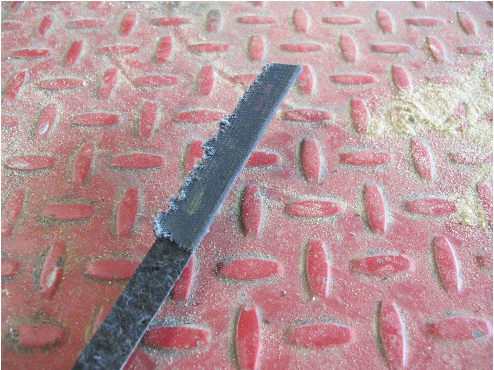
Photo 8 – View of damage to V-belt. Note: V-belt cut for removal (RH Photo)
